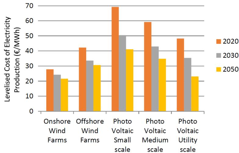
*Figure 1.3.* LCOE of RES used in Denmark for [Mathiesen et al., 2017]
