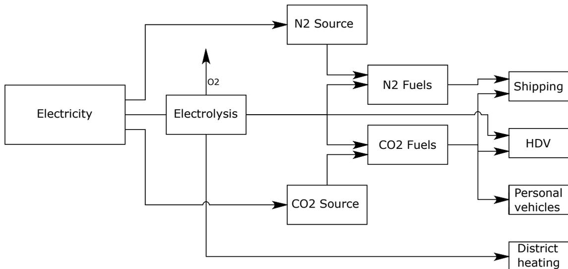
*Figure 6.1.* Overview of use cases for carbon and nitrogen based e-fuels
