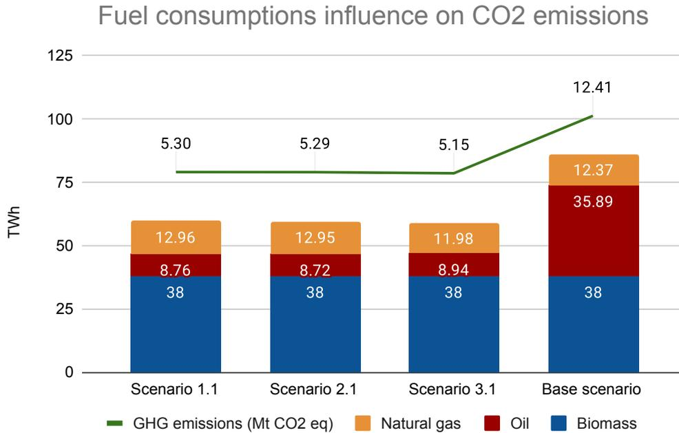
*Figure 8.7.* Fuel consumptions impact on the GHG emissions
