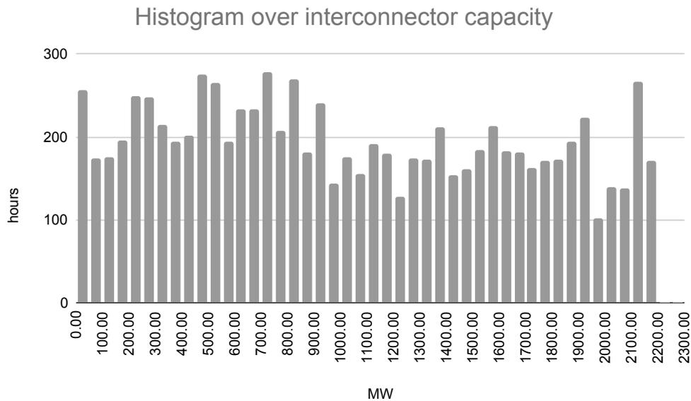
**Figure 7.1.** A histogram of the needed interconnector for all hours of the year
