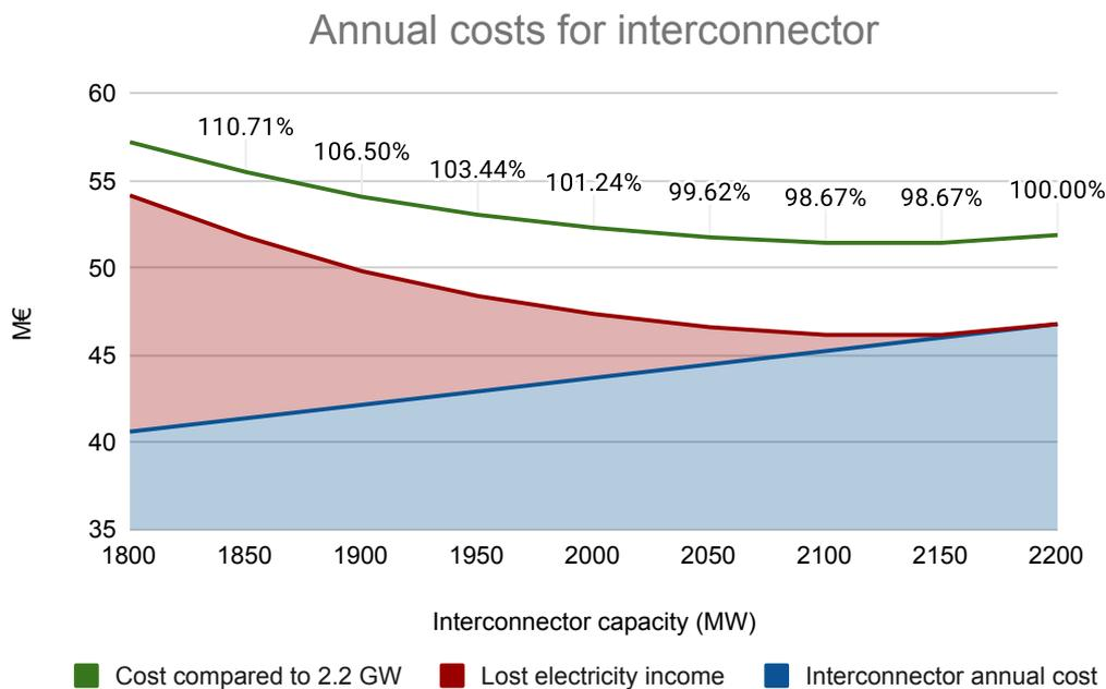
*Figure 8.1.* Annual interconnector costs with wind turbine down time included
