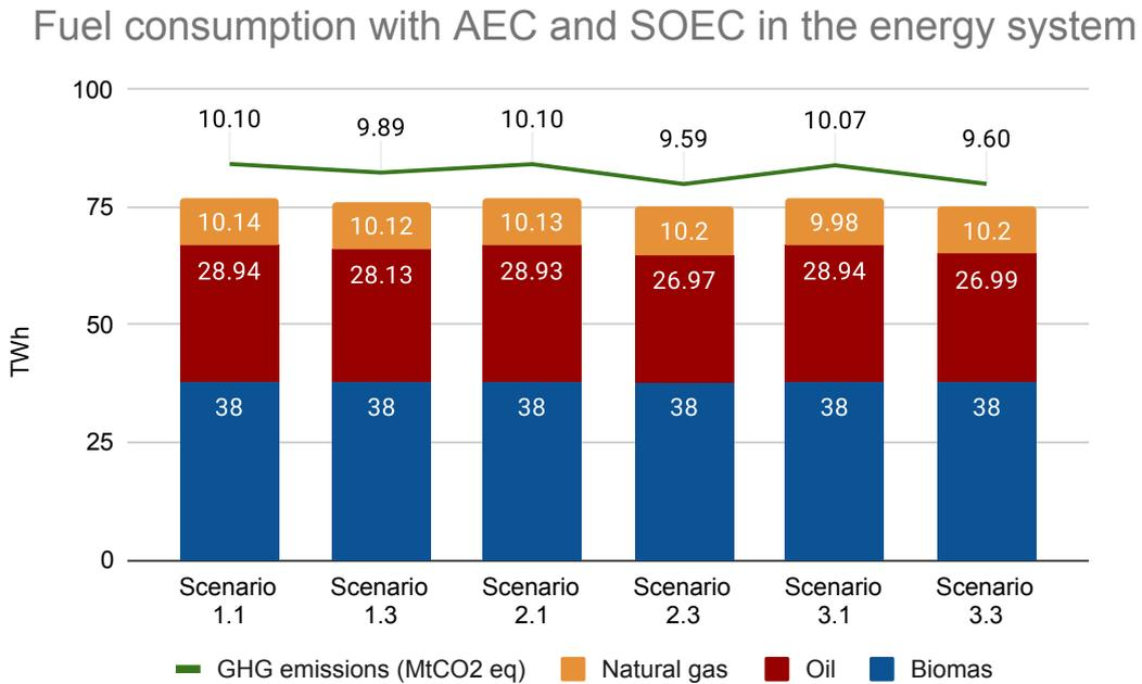
**Figure 8.10.** GHG emissions for 3 GW energy island with AEC and SOEC
