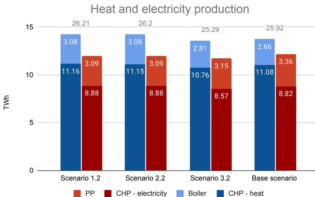
*Figure 8.6.* Annual heat and electricity production from Scenario X.2
