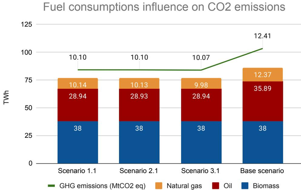
*Figure 8.4.* Fuel consumptions impact on the GHG emissions
