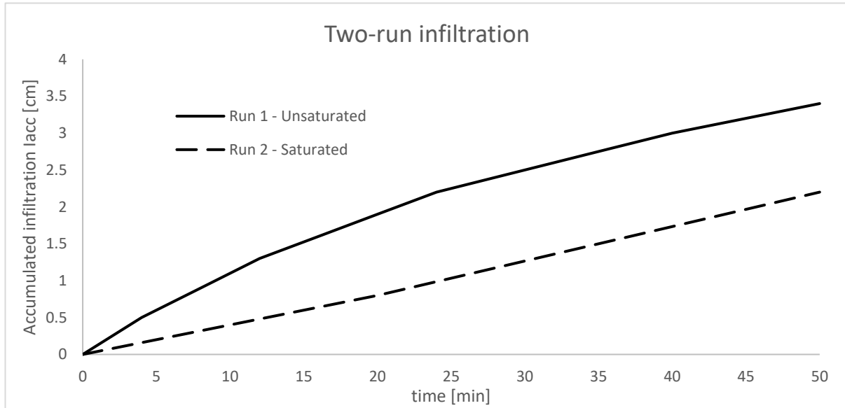
Figure 14 Assumed progress of accumulated infiltration versus time for a double ring infiltrometer experiment under unsaturated and saturated initial conditions. The differences in water infiltration can be seen – for the same duration in the same soil Run 1 is expected to produce a curved line, infiltrating more water than Run 2, which is characterized by its linearity.
