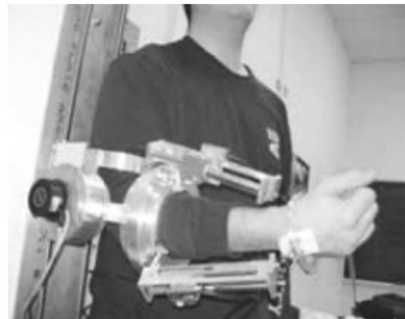
(b) Haptic exoskeleton designed for virtual tasks (Gupta and O'Malley, 2006)
