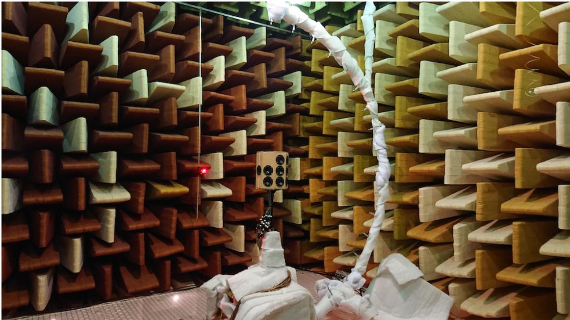
**Figure 7.10:** Picture of the setup for the 3D measurement of the sound radiation loudspeaker array.
