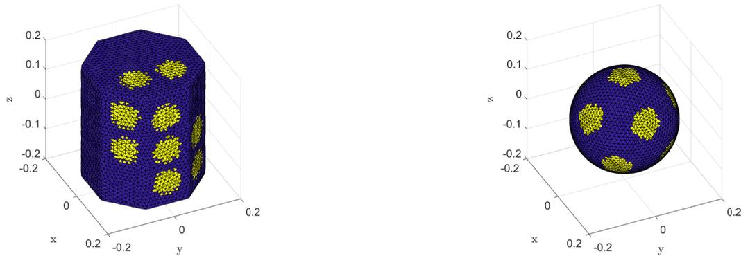
(a) Octagonal prism array with 12 non-uniformly placed loudspeakers
