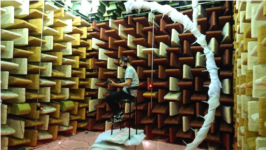
**Figure 4.7:** Picture of the setup for the 3D measurement of the sound radiation of the acoustic guitar. The guitarist is seated on a chair located on a turntable in the middle of an arch of microphones.
