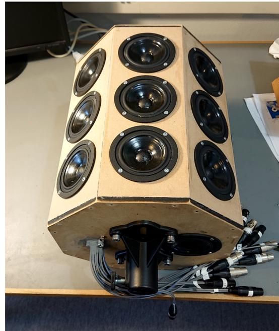
(b) The finished loudspeaker array from the front right side.
