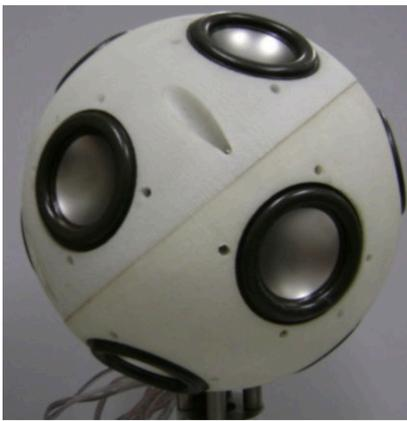
(d) The spherical loudspeaker array (12 drivers) by Pasqual. Figure from [43]
