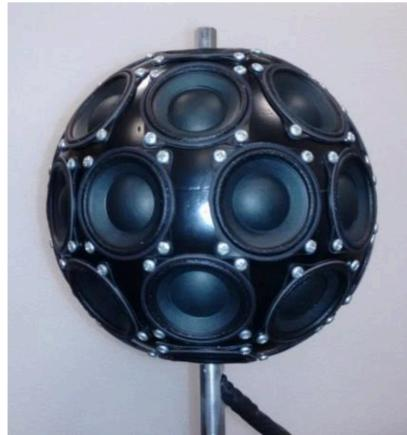
(e) The spherical loudspeaker array (32 drivers) by Farina *et al.*. Figure from [6]
