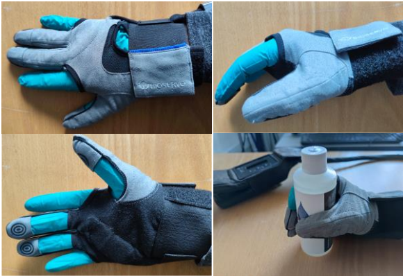
Fig. 1. Different views of the SEM TM Glove from Bioservo Technologies [27]. Top left, back view of the glove, top right, lateral view of the glove, bottom left frontal view of the glove, bottom right, glove while holding the bottle. The subject is also wearing a blue plastic glove to follow the coronavirus health guidelines. In the background of the bottom right picture the box containing the motor and controller of the glove is present.
