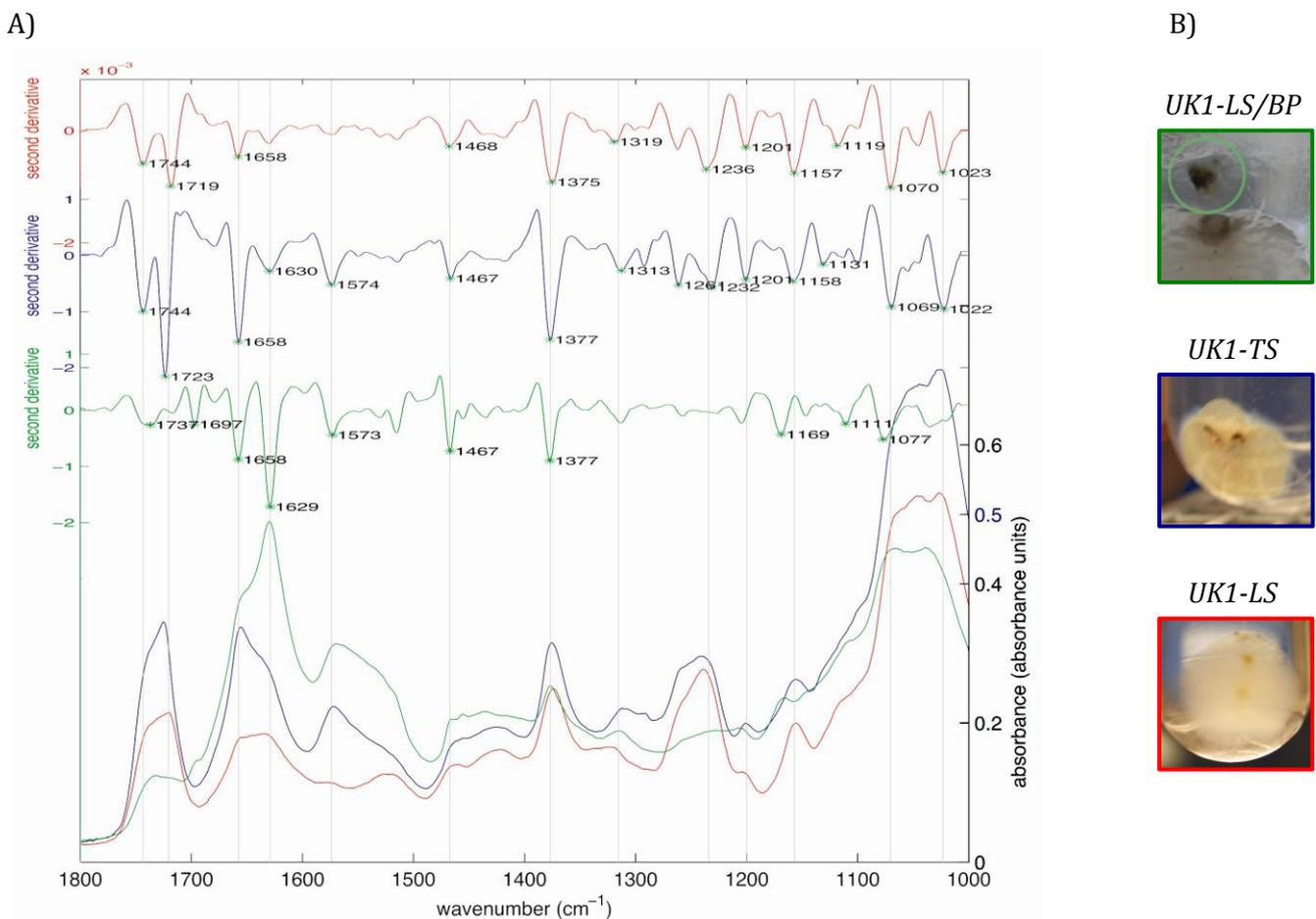
Fig. 7 FTIR of *UK1-LS/BP*, *UK1-TS* and *UK1-LS*.
