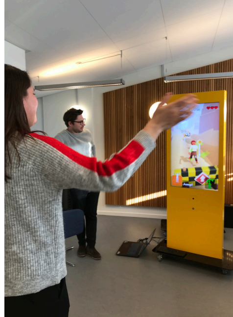
Picture 1: Shows the Rehaboo technology consisting of a yellow iron 'totem', a gaming computer, a large screen and a motion sensor. On the picture on the right you can see the totem in action.
