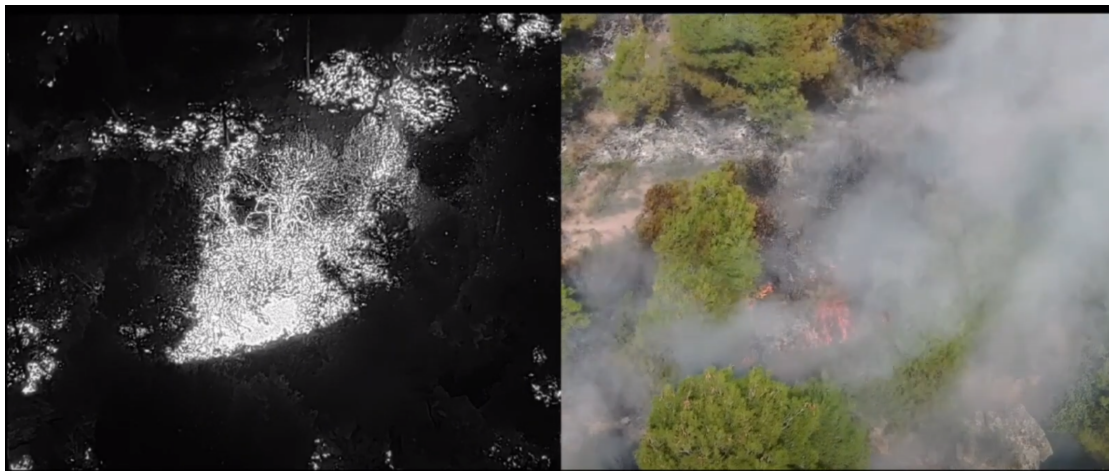
Figure 2.1: Image of a wildfire taken by a drone (DJI Matrice 300 using a Zenmuse H20T). The left side shows the Thermal channel which clearly displays the hot spots. On the right side the color image shows flames and smoke. While fire is clearly visible, locating this fire in the real world only based on this image would be very hard. Picture provided by Robotto.
