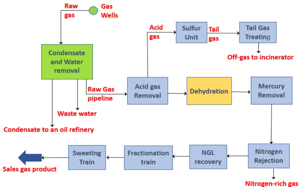
Figure 2. A typical onshore natural gas processing plant (Okafor & Ewrierhurhoma, 2020)
