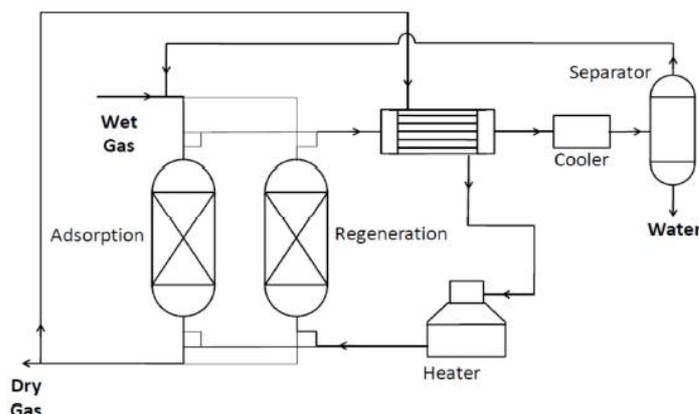
Figure 9. A typical process flow diagram for adsorption dehydration process [Reproduced from (Engineering & Harcourt, 2016).
