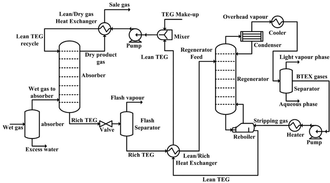
Figure 12. A typical process flow diagram for DRIZO process (Kong et al., 2018).
