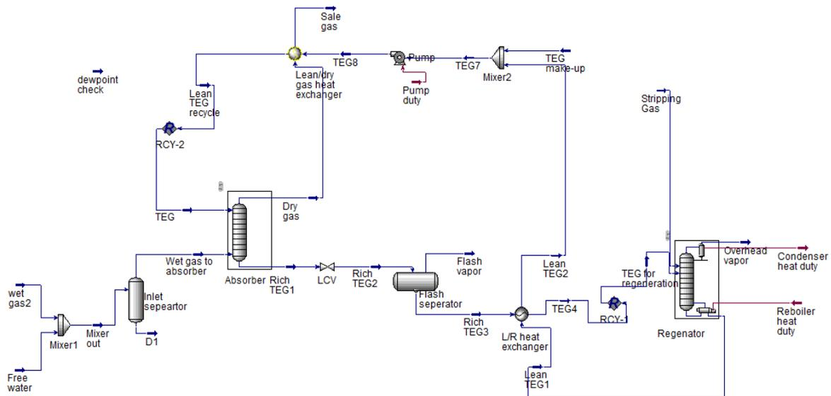
Figure 13: The HYSYS model of TEG dehydration unit.
