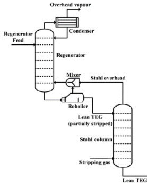
Figure 11. Stahl column (vapor flows directly into the bottom of the regeneration column (Kong et al., 2018).
