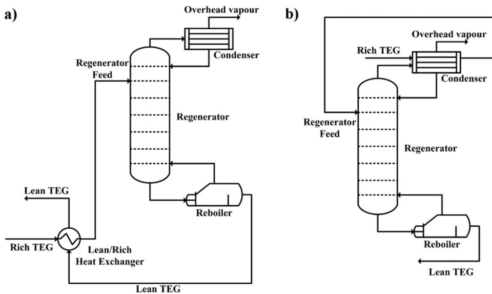
Figure 7. The two different heating configurations for water-rich TEG for regeneration a) Heating by an overhead condenser b) Heating by a glycol-to-glycol heat exchanger [reproduced from (Rahimpour et al., 2013)(Netusil & Dittl, 2011).
