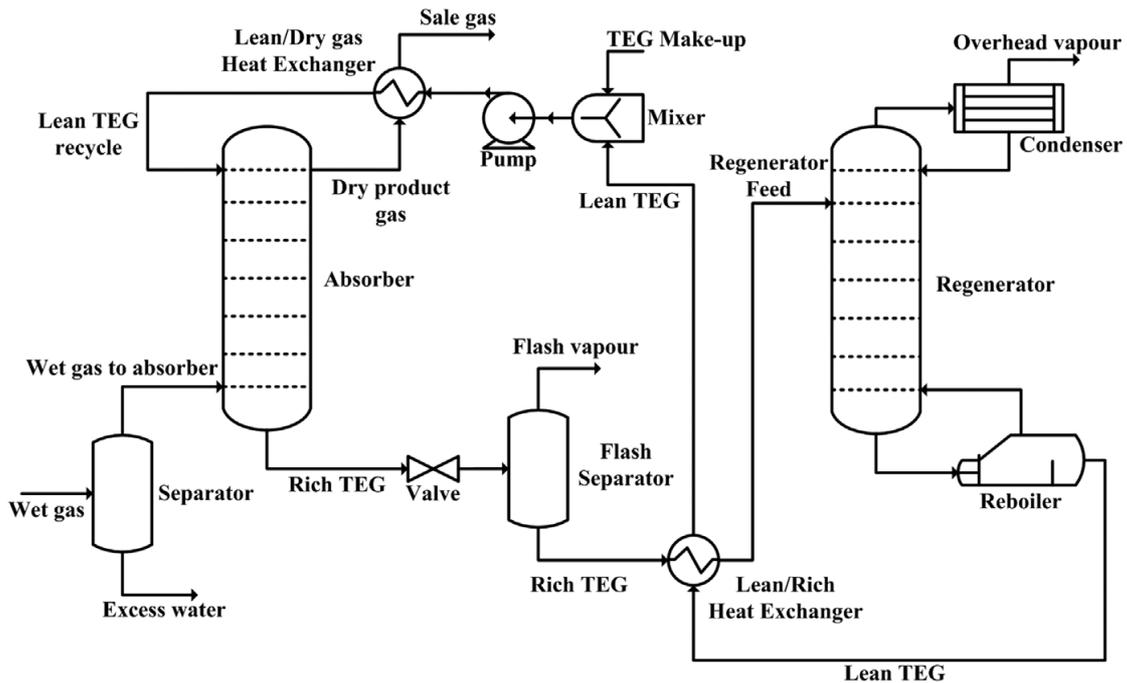
Figure 5. A typical process flow diagram for absorption dehydration process (Øi, 2003).
