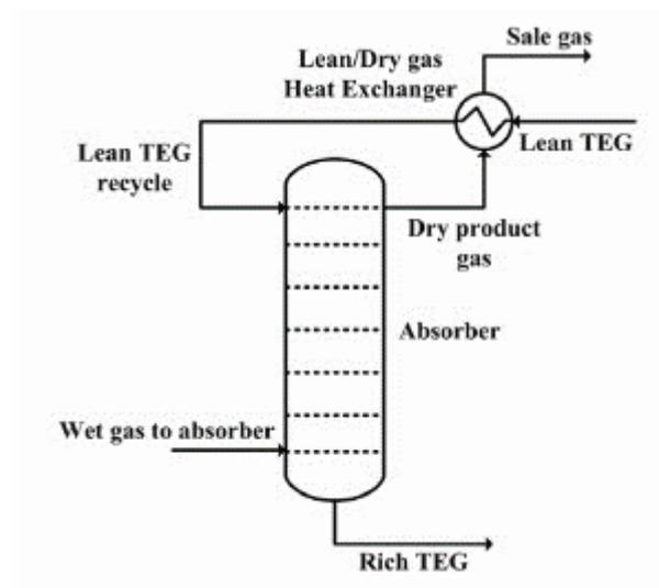
Figure 8. The water-lean TEG before entering to absorber unit cooling by heat exchange with dry gas product gas (Díaz Rincón et al., 2016) (Rahimpour et al., 2013)(Netusil & Dittl, 2011).
