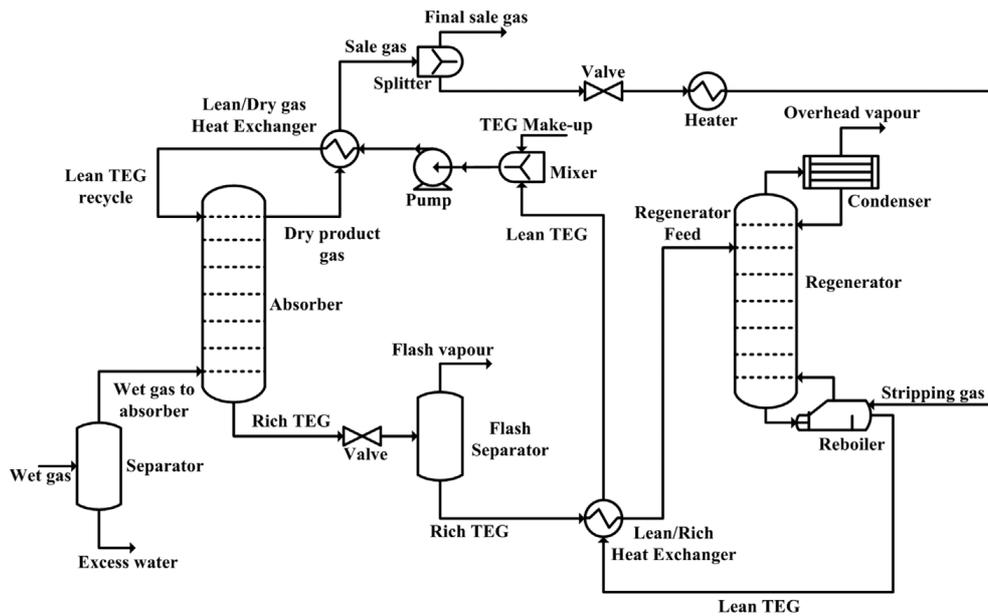
Figure 10. Stripping gas process using the injection of a portion of dry product gas (sale gas) into the regeneration column (Kong et al., 2018).
