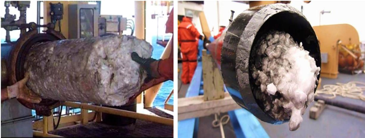
*Figure 1. Hydrate formation in transmission line (Sajjad, 2018).*
