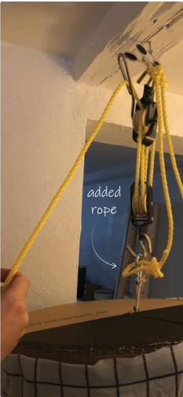
III. 141. 1:1 mockup testing of adjustable rope that stops the hoisting system
