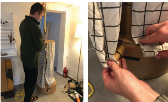
III. 136. 1:1 mockup testing of aligning air valve on cover with air pump on box
