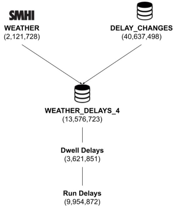
*Figure 6. Data Collection Process. From original weather and delay observations to one table entitled weather\_delays\_4 which was processed in SQL and used for regression modelling in R Studio*
