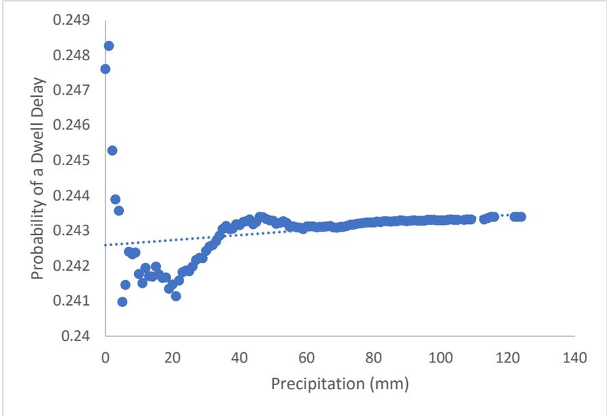
Figure 10. The Probability of a Dwell Delay for a Given Sum of Precipitation over 7 Days
