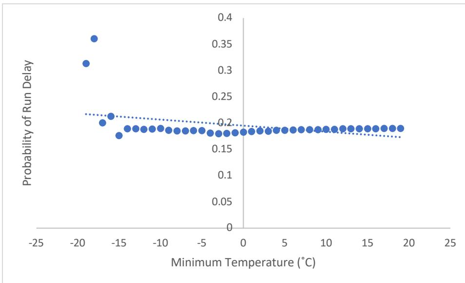
Figure 26 The Probability of a Run Delay for a Given Minimum Temperature over 14 Days
