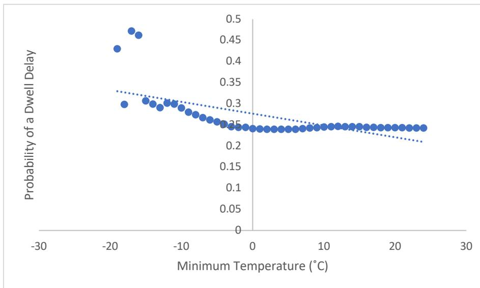
Figure 19 The Probability of a Dwell Delay for a Given Minimum Temperature over 1 Day
