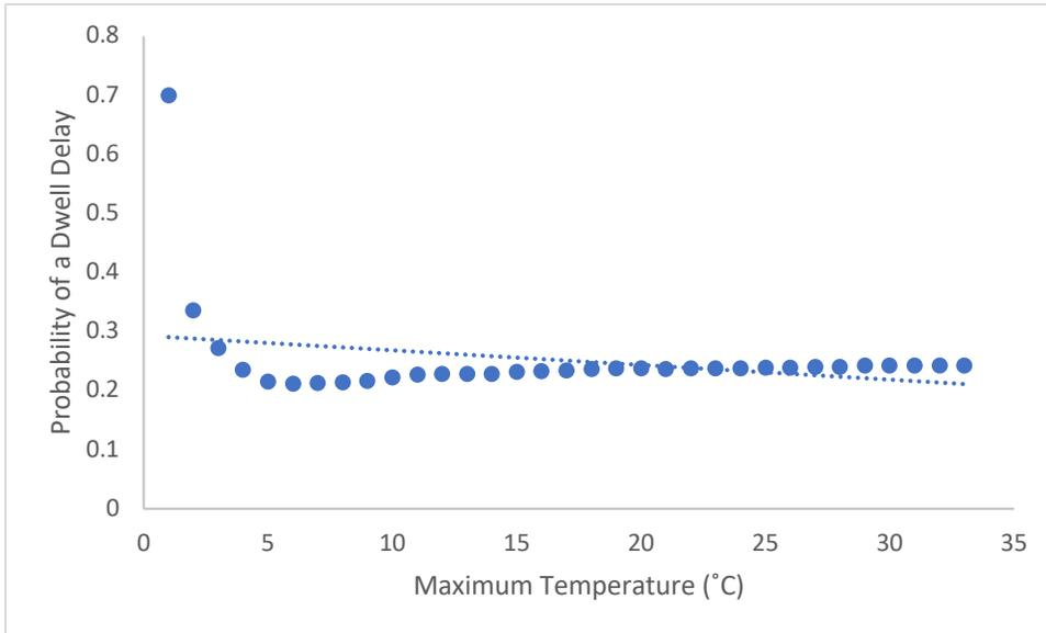
Figure 33 The Probability of a Dwell Delay for a Given Maximum Temperature over 28 Days
