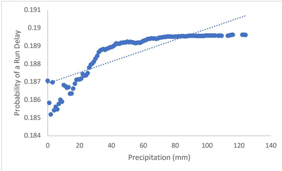
Figure 15 The Probability of a Run Delay for a Given Sum of Precipitation over 7 Days
