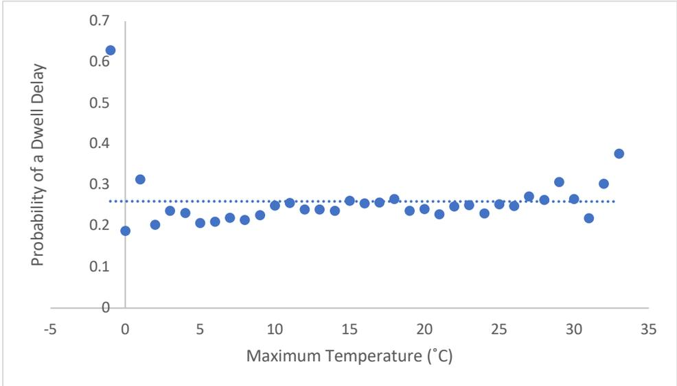
Figure 32 The Probability of a Dwell Delay for a Given Maximum Temperature over 21 Days
