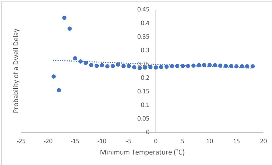
Figure 22 The Probability of a Dwell Delay for a Given Minimum Temperature over 21 Days
