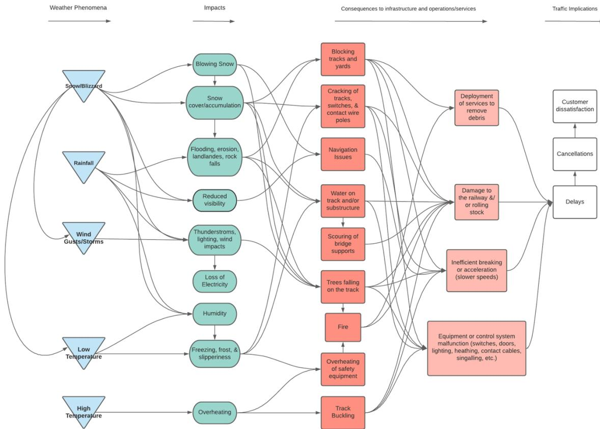
Figure 8. “Different weather phenomena and their impacts, consequences, and traffic implications for railways. Figure adapted from: Kreuz, et al., 2012” and further adapted to fit this region (Ochsner, 2021).
