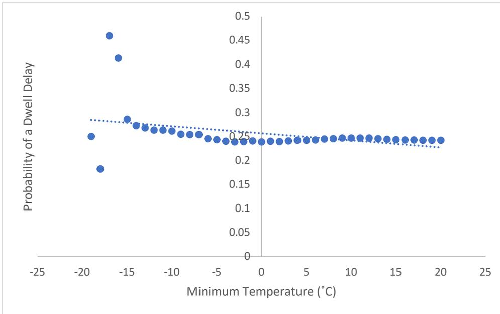
Figure 20 The Probability of a Dwell Delay for a Given Minimum Temperature over 7 Days
