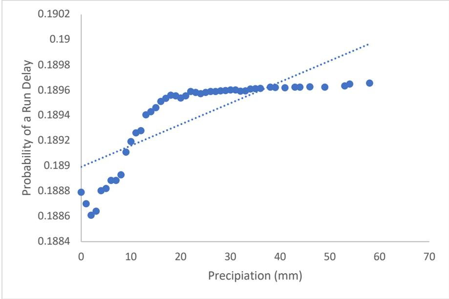
Figure 14. The Probability of a Run Delay for a Given Sum of Precipitation over 1 Day
