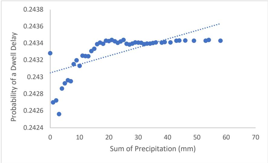
Figure 9. The Probability of a Dwell Delay for a Given Sum of Precipitation over 1 Day
