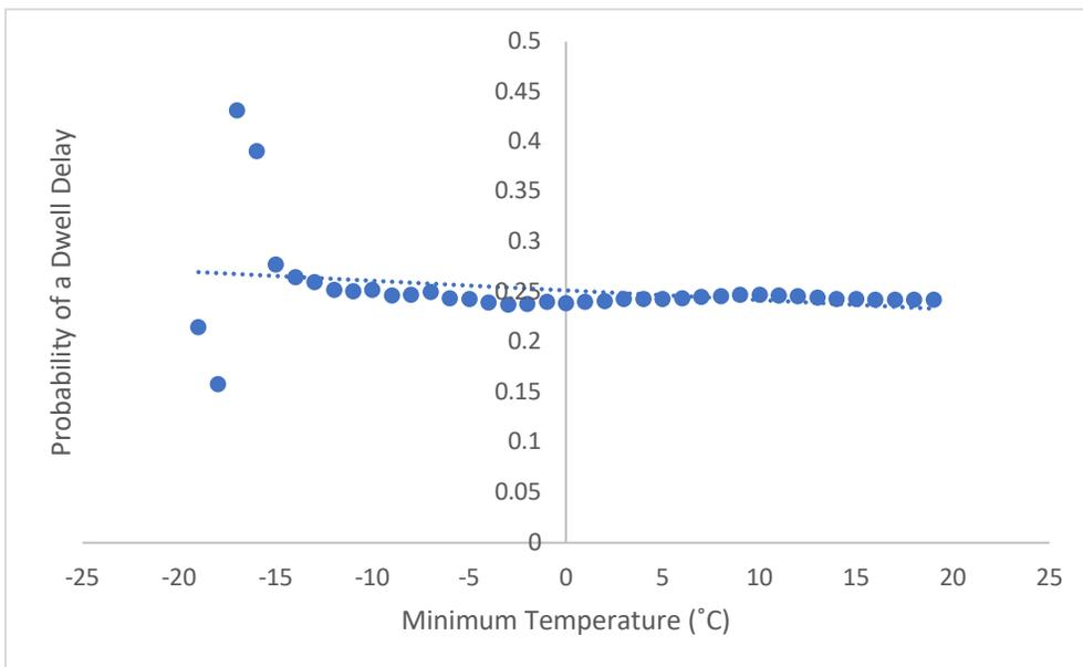
Figure 21 The Probability of a Dwell Delay for a Given Minimum Temperature over 14 Days
