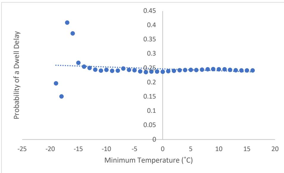
Figure 23 The Probability of a Dwell Delay for a Given Minimum Temperature over 28 Days
