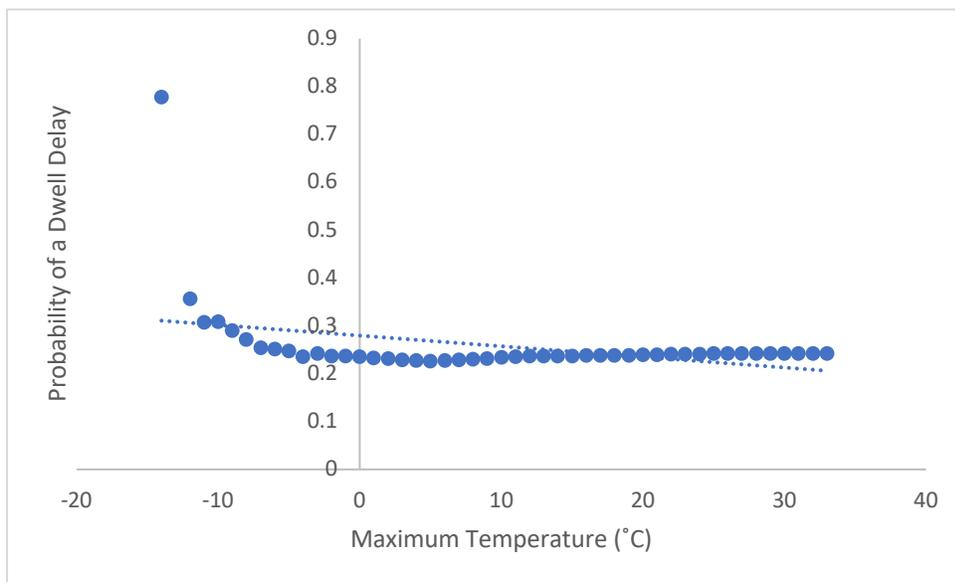
Figure 29 The Probability of a Dwell Delay for a Given Maximum Temperature over 1 Day
