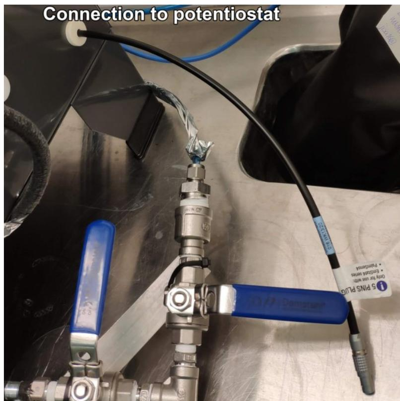
**Figure B.6:** Connection port which tightly fit the 5 pin cable from the PalmSens4 potentiostat. During electrochemical experiments the potentiostat unit was placed outside the glovebox.
