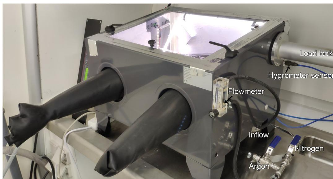
**Figure B.1:** Outside view where the gloves are sticking out due to a slight overpressure.
