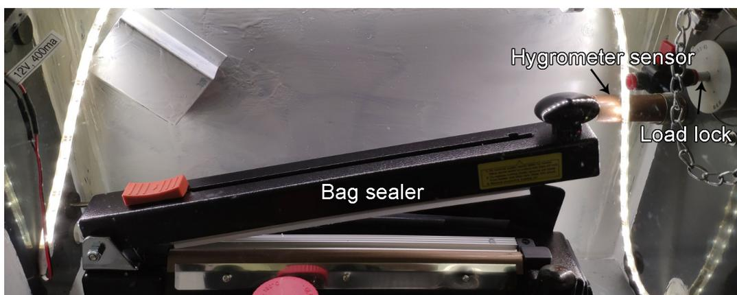
**Figure B.3:** Inside view with bag sealer, hygrometer sensor, and load lock sealed with a rubber stopper and a valve.
