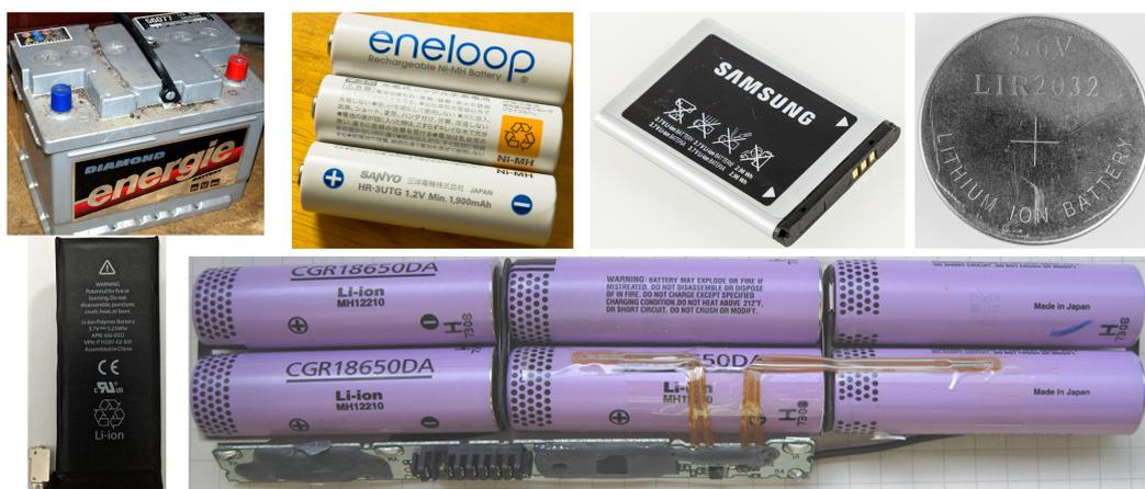
**Figure 2.4:** Different types of secondary batteries. First row from left to right: Lead-acid automotive battery 12 V, HR6 Ni-MH rechargeable 1.2 V, prismatic Li-ion 3.7 V, and Li-ion button cell type LIR2032 3.6 V. Second row from left to right: Li-ion polymer pouch 3.7 V, and CGR18650 cylindrical Li-ion batteries with LiNiCoMnO<sub>2</sub> cathode, 3.6 V, assembled into a laptop battery pack operating at 10.8 V. For image references see [27].
