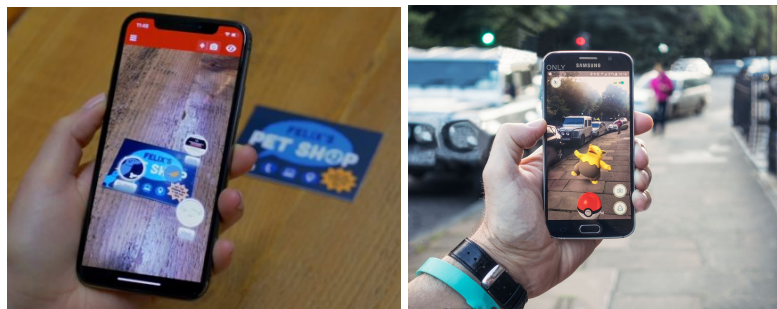
Figure 2.2: (left) Example of marker-based AR. Business card used for recognition. (right) Example of marker-less AR (Pokemon GO). GPS and surface detection used for proper projection of augmented objects.
