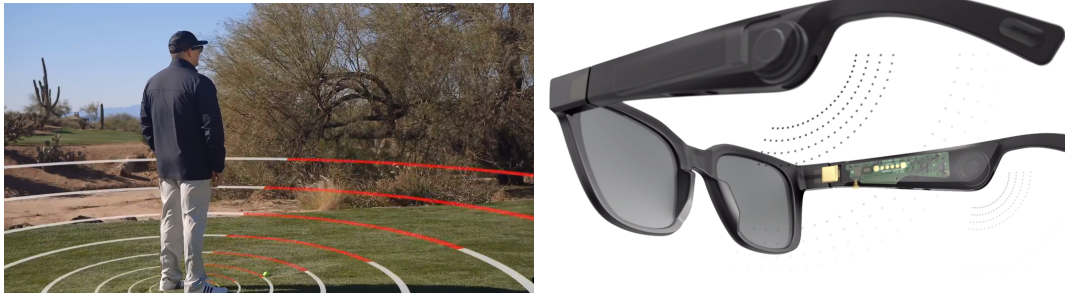
Figure 2.11: (left) User attempting to locate the correct direction of the green through an obstruction, wearing the Bose Frames. (right) The Bose Frames. The speakers located in the arms of the frames visibly affect the form-factor.
