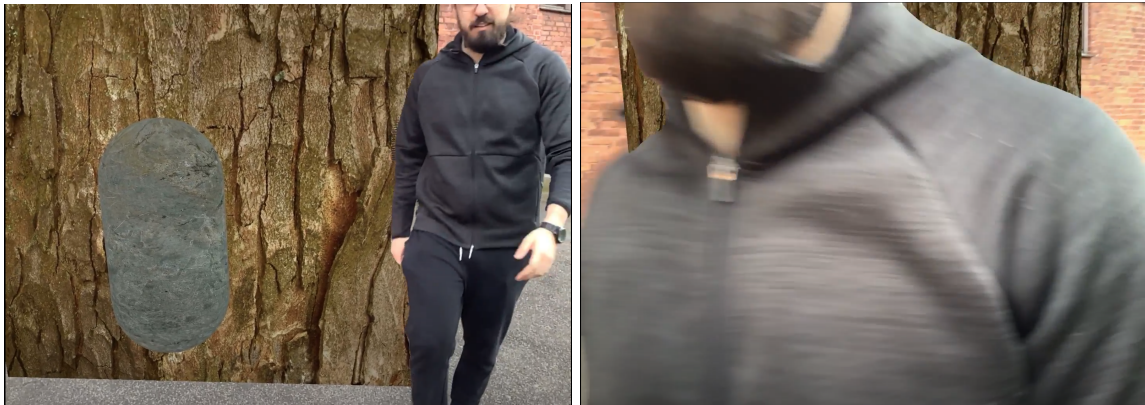
Figure 5.10: Person walking “around” objects and into the foreground. Notice the difference in stenciling, contrast and blurriness of the person vs. the wall between both images - Virtual objects retain clarity while the person is blurred when moving at close proximity.
