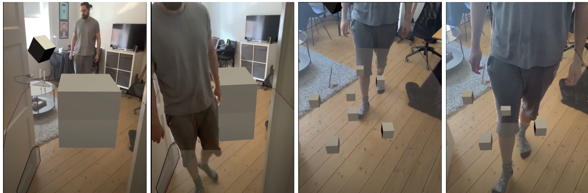
Figure 5.8: Early occlusion test-scenario using surface detection and a calibrated environment (transparent layer).
