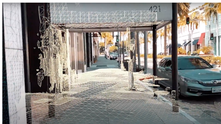
Figure 2.13: Reach and speed test of LiDAR scanner on iPad Pro 2020 [31].
