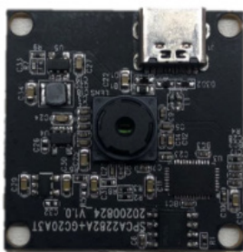
83. Webcam module on PCB (Webcam, n.d.)
