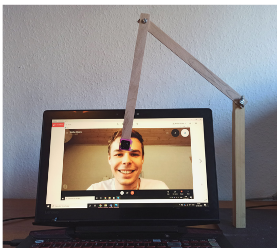
35. Prototype, webcam on swing-arm
