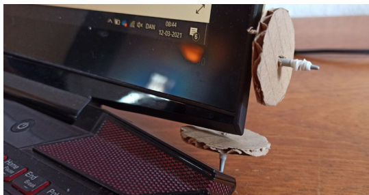
41. Prototype, webcam with wheel-controller
