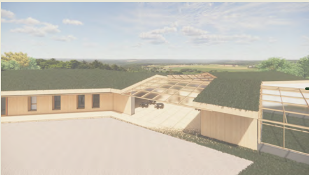
7. Skylights of polycarbonate exploiting the daylight without any direct sun
