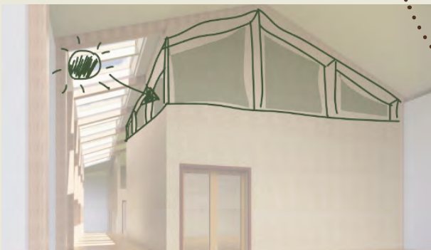
III. 49. Improving daylight by adding interior windows
