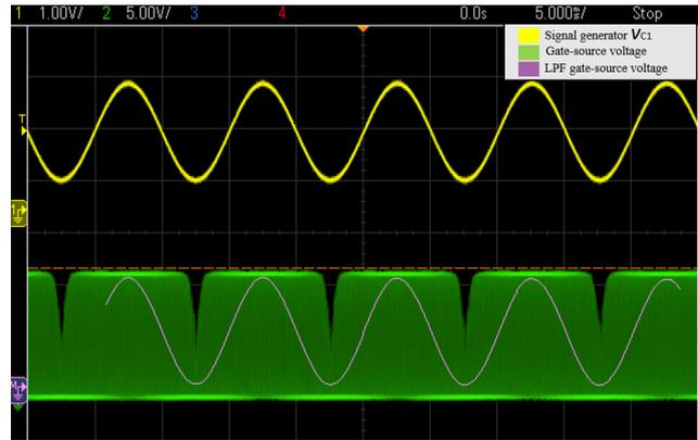
**Figure 5.14:** Gate-source voltage applied to top MOSFET of second leg in order to mitigate ripple component of low-voltage feedback signal  $v_{C1}$
