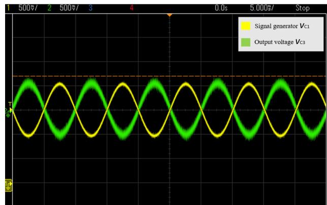
**Figure 5.20:** Resulting output voltage  $v_{C3}$  controlled to mitigate a low-voltage feedback signal  $v_{C1}$  equivalent to a reduced load of 150 W, across a larger time interval
