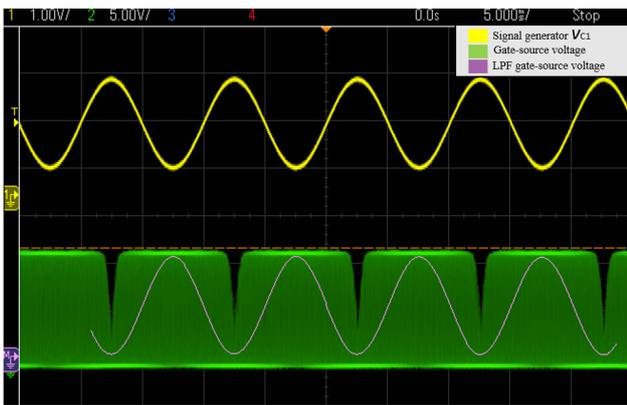
**Figure 5.13:** Gate-source voltage applied to top MOSFET of first leg in order to mitigate ripple component of low-voltage feedback signal  $v_{C1}$
