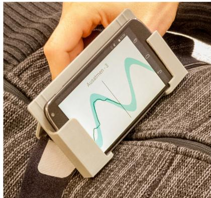
**Figure 2.6:** Breathing Mentor : Abdominal positioning of device containing app
