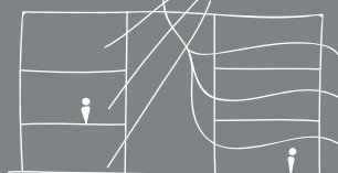
An atrium in the middle of the building for light and ventilation and connects the different floors.
