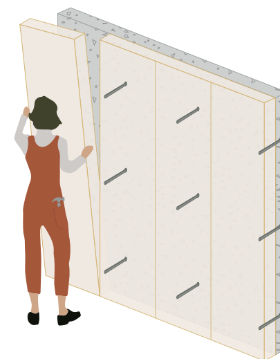
4 Insulation material is separated from the concrete
