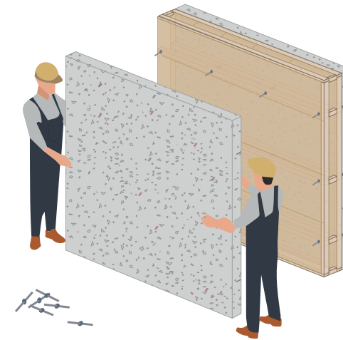
2 The exterior element is carefully detached by removing the plastic connectors. The connectors can be recycled
