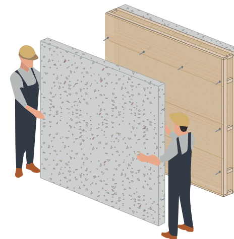
6 The new down-cycle concrete elements are placed on the exterior and fastened with connectors
