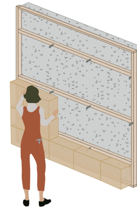
4 Straw insulation panels are removed and left on the fields to decompose naturally
