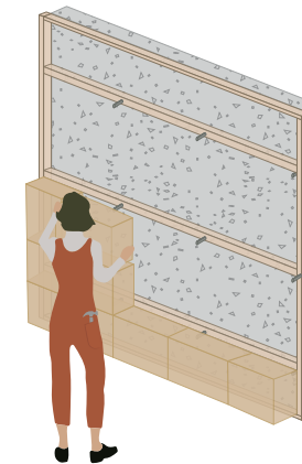
4 Straw insulation battens are secured in the wooden construction
