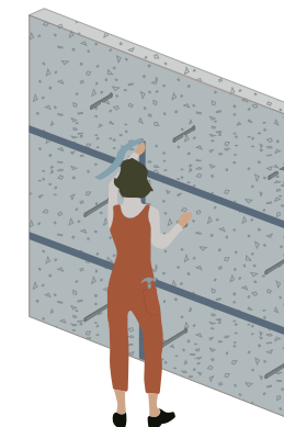
6 The paper vapor barrier is taken down by removing the airtightness tape and can be reused elsewhere
