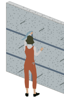
2 A paper vapor barrier is fastened with air-tightness tape
