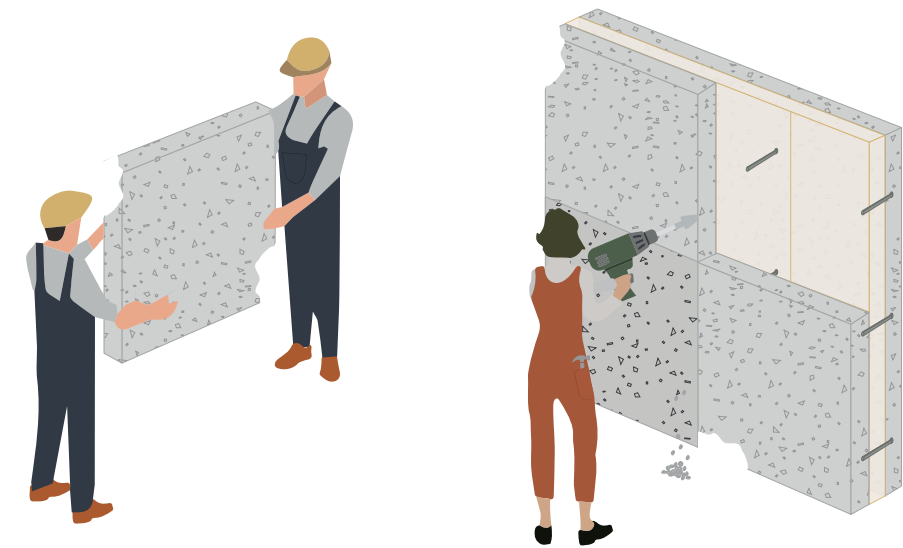
2 A simple tool can separate the concrete from the connectors and be taken down in small elements
