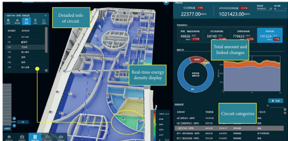
Figure 21 Real time visualisation of energy consumption in a hospital through DT implementation (Peng, et al., 2020)
