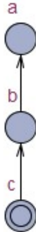
Figure 1.2: Example of a basic reduction. This simple model starting in c where it can only move to b then a can have the b location removed so we simply go straight to a as long as b is not a part of the query.
