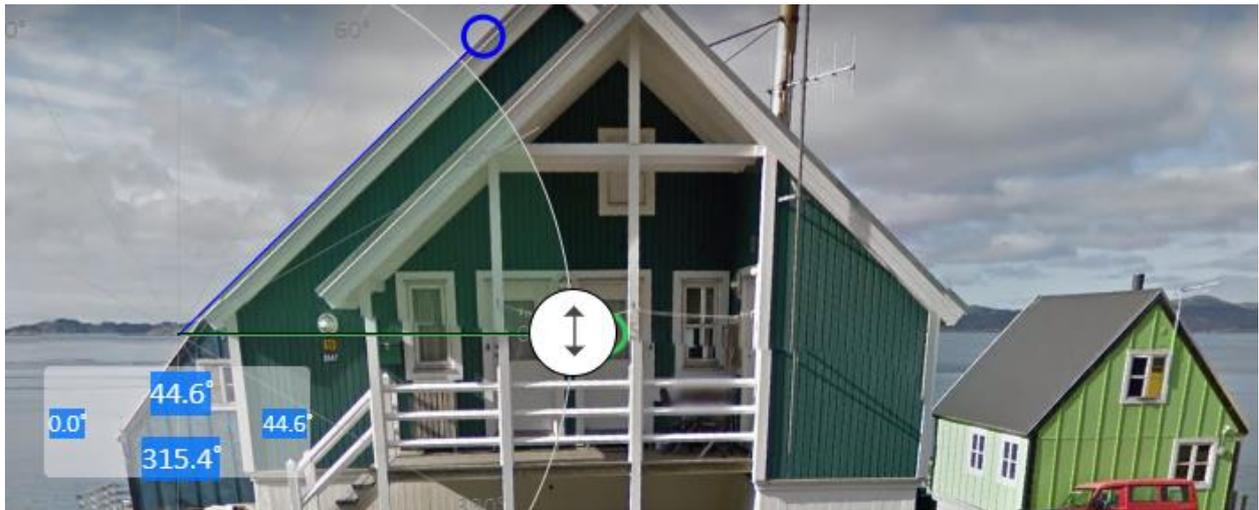
Figure 12 Measuring the roof angle in Google Street View
