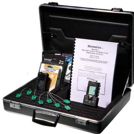
Figure 11 A portable system of sensors and instrumentation for static and dynamic measurements in a clinical setting. Source: Medicalexpo.com
