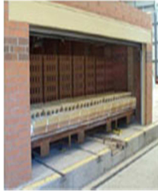
a. Extruding a brick column b. Brick stacks ready for fire c. Firing bricks in kiln
