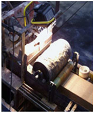
a. Extruding a brick column b. Brick stacks ready for fire c. Firing bricks in kiln
