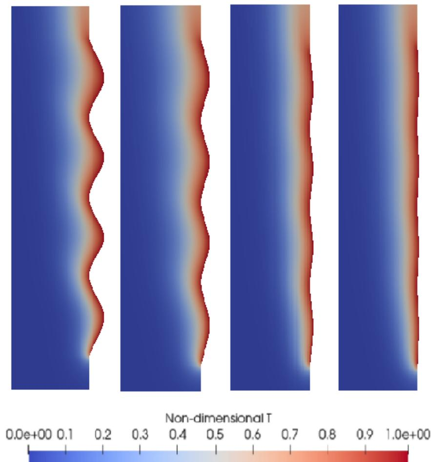
**Figure 5.2:** *Non-dimensional temperature field of the four geometries studied in the first investigation. From left to right, the  $L/d$  value is respectively equal to 5, 10, 20, 40.*
