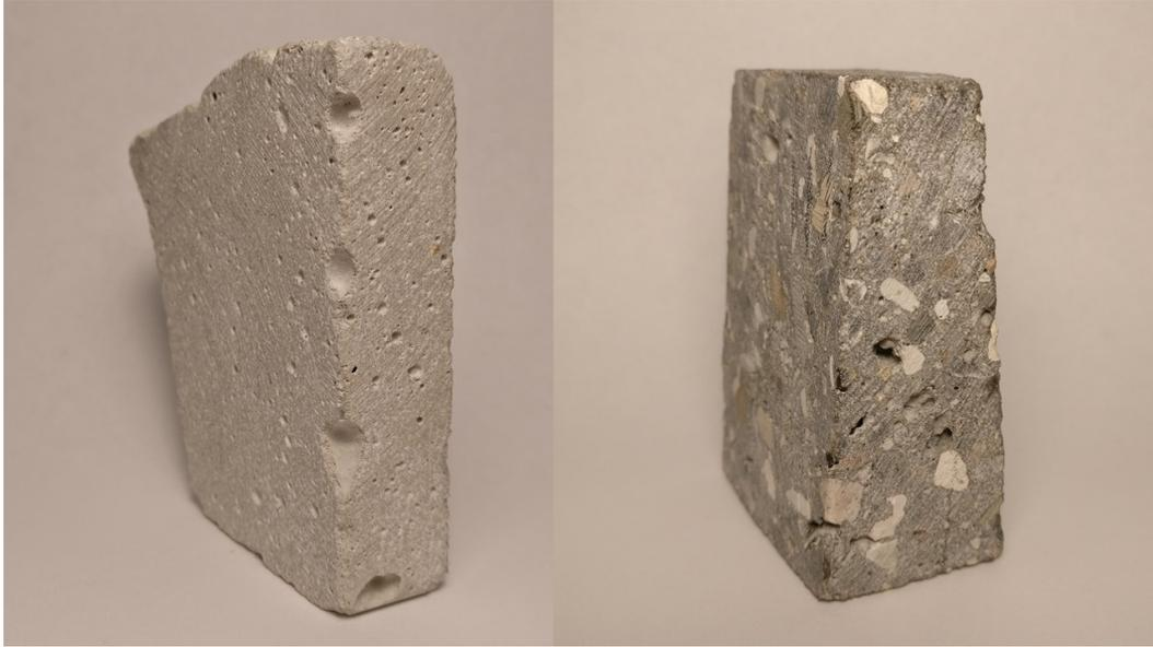
**Figure 4.1:** Sample ASC1 (left) and STDC1 (right). Both samples are presented after being ground in order to remove the carbonated layer and expose an unreacted surface.
