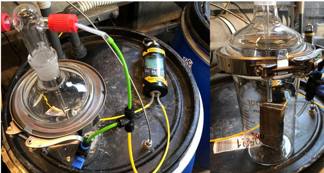
**Figure 4.6:** Reactor setup for the H<sub>2</sub>S uptake rate measurements of ASC2 and STDC3.
