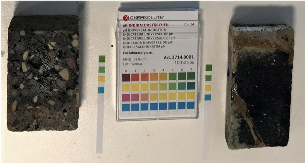
**Figure 4.7:** Samples ASC2 (left) and STDC3 (right) prior to the  $H_2S$  oxidation test in the reactor after being 2 months in the incubator.
