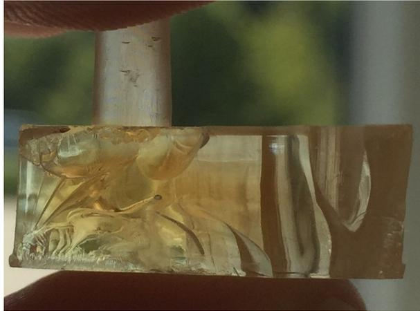
Figure 7.3: Side view of the cross sectional area of the droplet generator after approximately 2 months in acetic acid.
