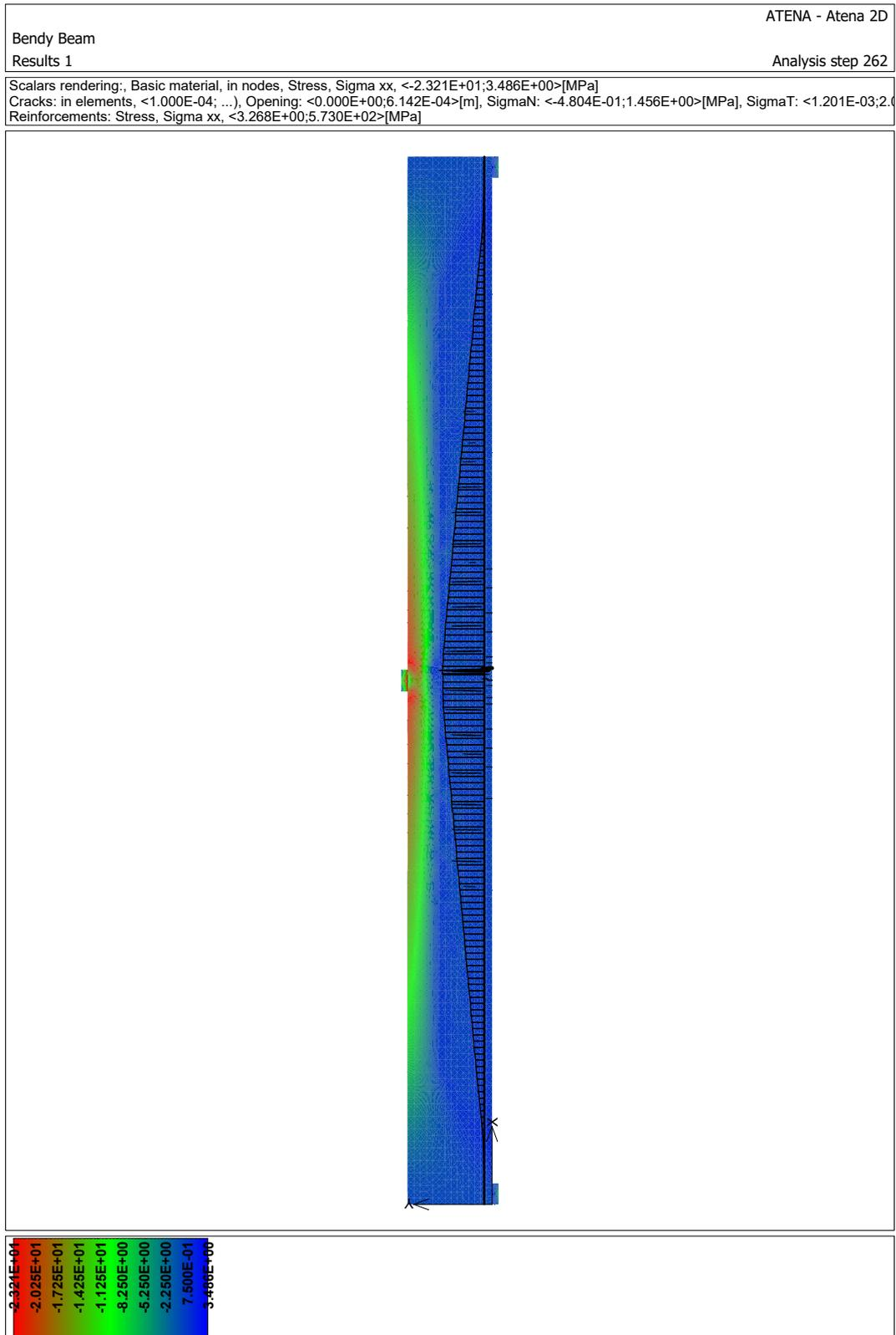
Figure B.0.3: Rectangular beam Sample no. 3.
