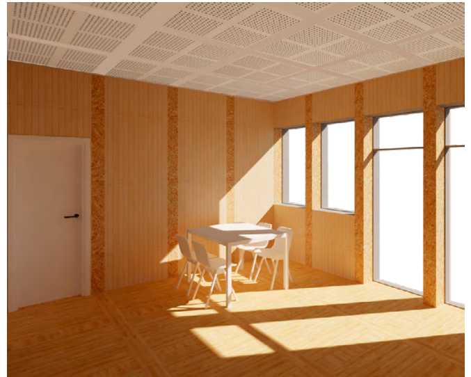
Illu 219: Pine, particle board, bamboo and gypsum Daylight factor: 3,7% Reverberation time average 125-4000 Hz: 0,5s
