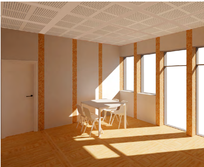
Illu 220: Gypsum, particle board, bamboo and gypsum Daylight factor: 3,8 % Reverberation time average 125-4000 Hz: 0,5s
