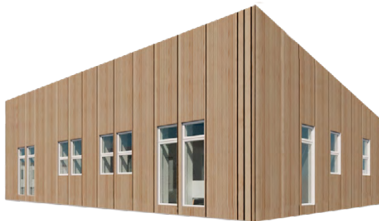
Illu 270: Natural ventilation 2. Mullions placed in the middle of the small windows
