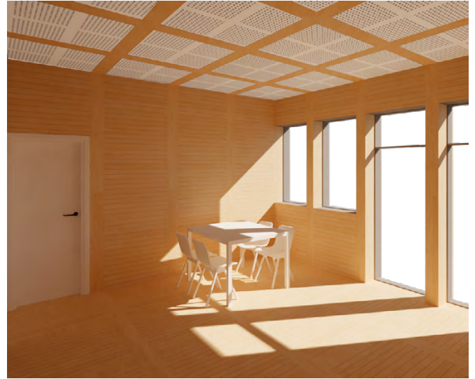
Illu 223: Pine, pine, pine and gypsum Daylight factor: 3,7% Reverberation time average 125-4000 Hz: 0,5s
