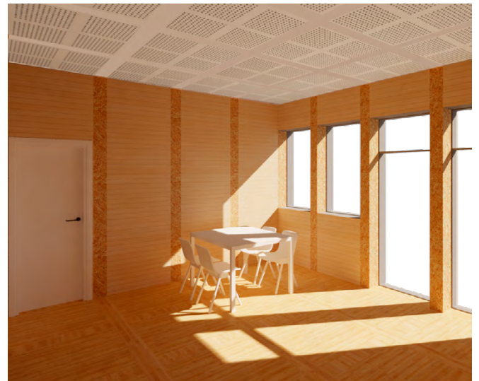
Illu 221: Pine, particle board, bamboo and gypsum Daylight factor: 3,7% Reverberation time average 125-4000 Hz: 0,5s
