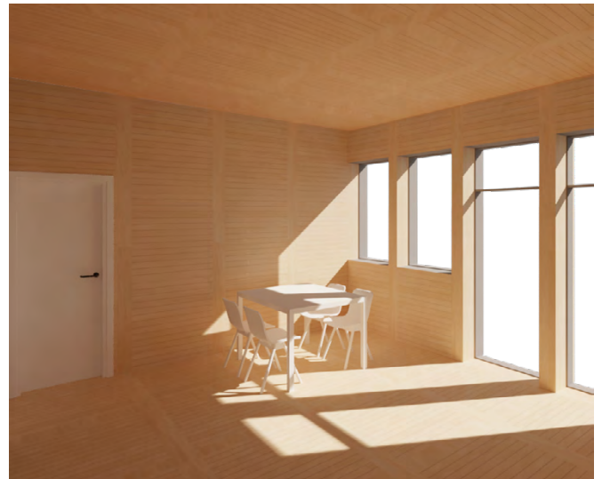
Illu 225: Pine, pine, pine and pine Daylight factor: 3,6% Reverberation time average 125-4000 Hz: 0,9s
