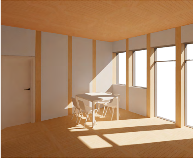
Illu 222: Gypsum, pine, pine and pine Daylight factor: 3,8% Reverberation time average 125-4000 Hz: 1,0s
