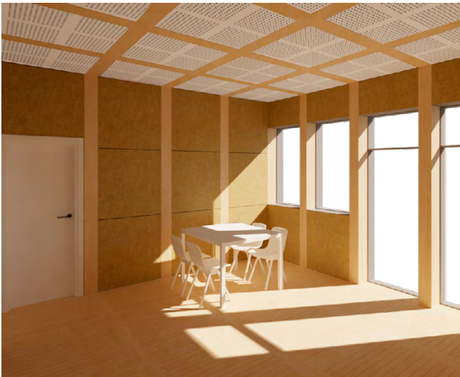
Illu 224: Clay, pine, pine and gypsum Daylight factor: 2,7% Reverberation time average 125-4000Hz: 0,4s
