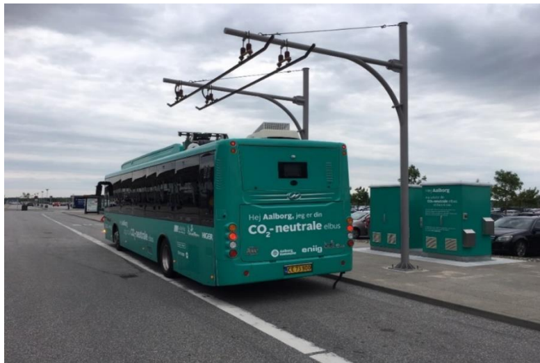
Figure 20. Super capacitor-based electric bus in Aalborg (Pedersen, 2019)
