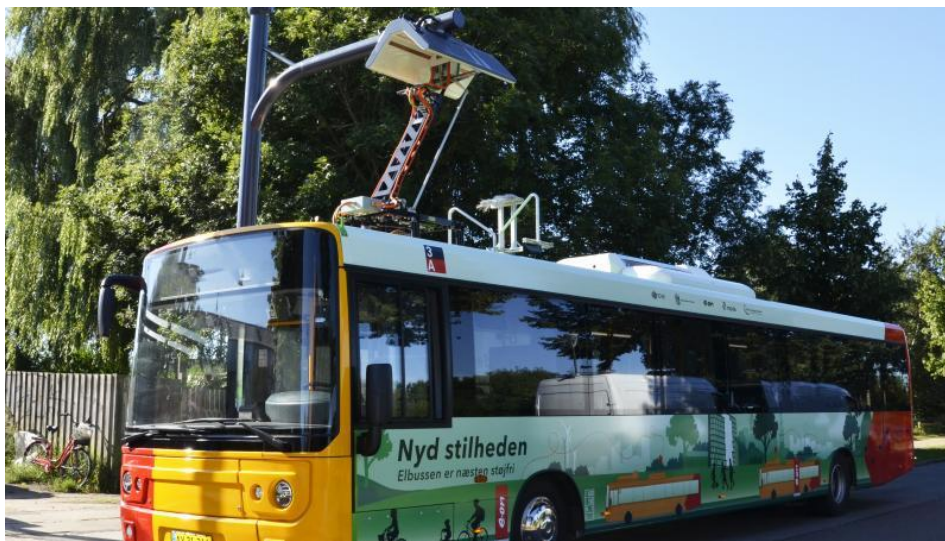
Figure 16. An electric bus in Copenhagen, charging through a pantograph- Terminal charging (Godske, 2017 c)
