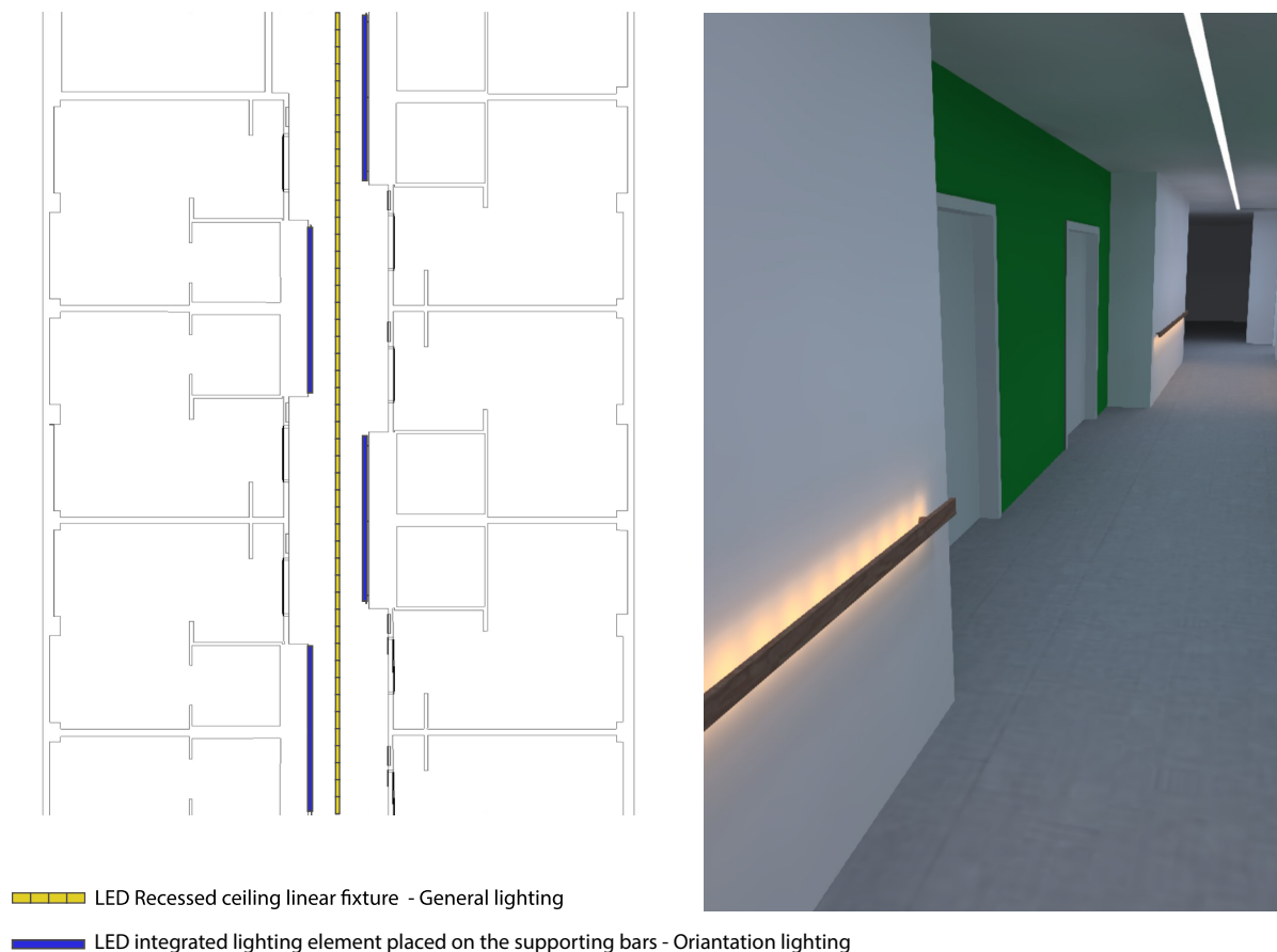
Figure 26: Lighting design for hallways - 2nd proposal
