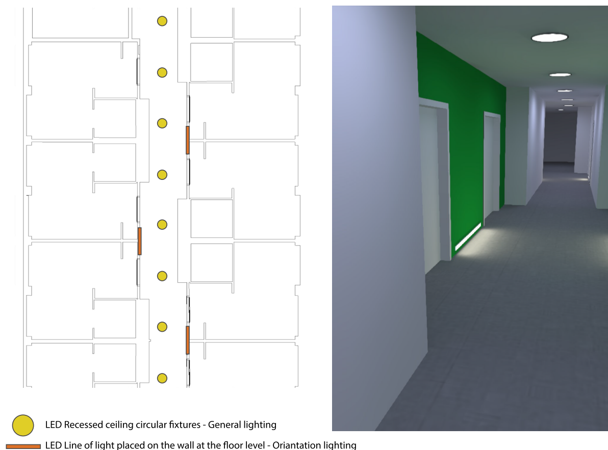
Figure 25: Lighting design for hallways - 1st proposal
