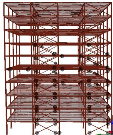
Figure 5.60: Damages occurrence in YZ plane, (final state)
