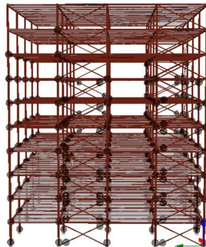
Figure 5.67: Damages occurrence in YZ plane, (final state)
