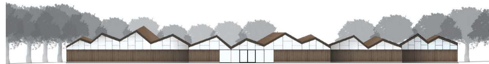
III.180 North facade with wood cladding (vertical wood lamellas)
