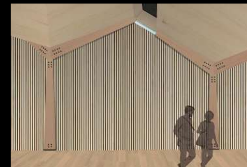
III.215 Wood lamellas (pinewood) on walls, wood boards on ceiling (pinewood), parquet floor and light columns
