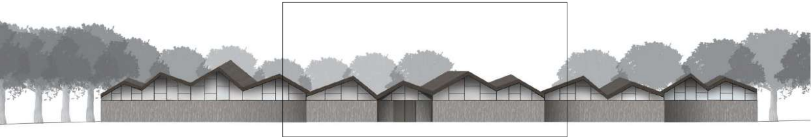
III.184 North facade with a vertical brick base that continues around the corners of the displaced entrance
