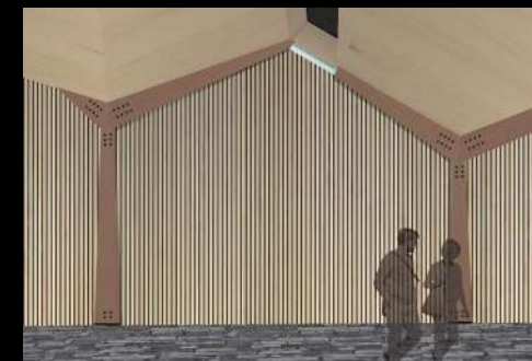
III.213 Wood lamellas (pinewood) on walls, wood boards on ceiling (pinewood), stone floor and dark columns
