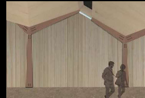
III.211 Wood lamellas (pinewood) on walls, wood boards on ceiling (pinewood), rammed earth floor and dark columns
