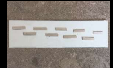
III.103 Materials on the floor used for guiding people forward in the right directions
