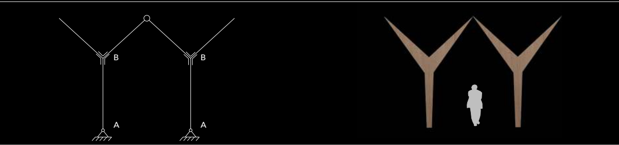
III.121 A: Hinge B: Fixed connection (static determinate)
