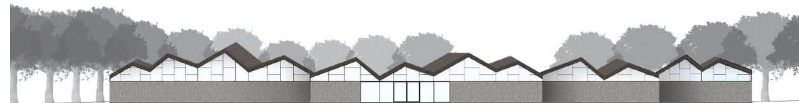
III.182 North facade with vertical bricks
