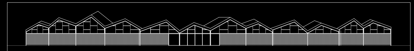
III.173 Investigation 5: North facade with a clear division between the base and the roof with the glass section in between with both horizontal and vertical glazing bars 1:500
