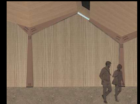
III.210 Case 4: Microperforated panels on walls, wood boards on ceiling, rammed earth floor
