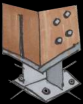
III.140 Column bolted to metal timber connector type 1
