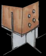
III.141 Column bolted to metal timber connector type 2
