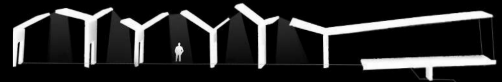
III.99 Section AA: Daylight entering the skylights at day
