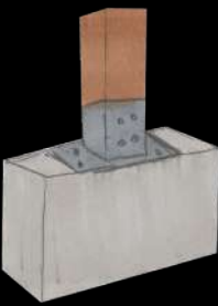
III.135 Column inserted in metal shell bolted to firm ground
