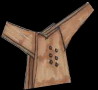
III.127 The column is divided into two pieces placed on each side of the beams
