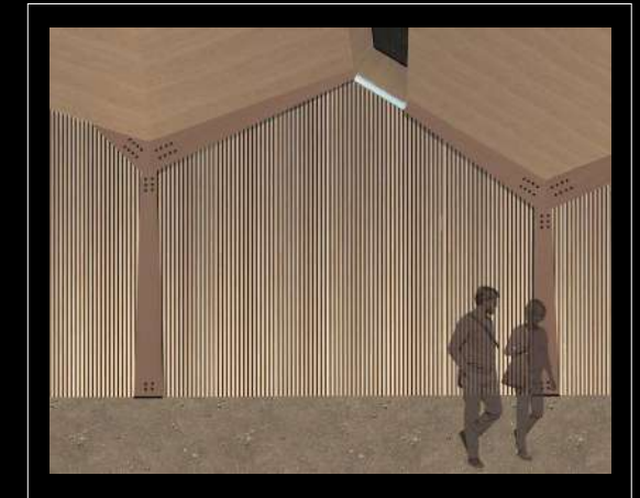
III.208 Case 2: Wood perforated lamellas (oak) on walls, wood boards on ceiling, rammed earth floor
