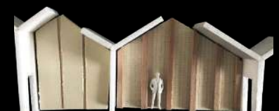
III.106 Materials used to indicate a distance within the room through the panels with the same width (left) or through regular placed columns (right)
