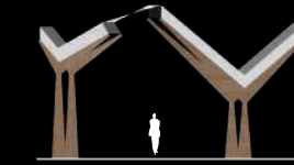
III.150 Front columns have a wider span - section
