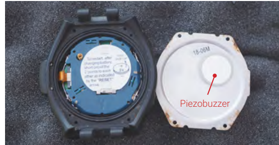
ill. 102 piezoelectric buzzer in Salvimar One dive watch
