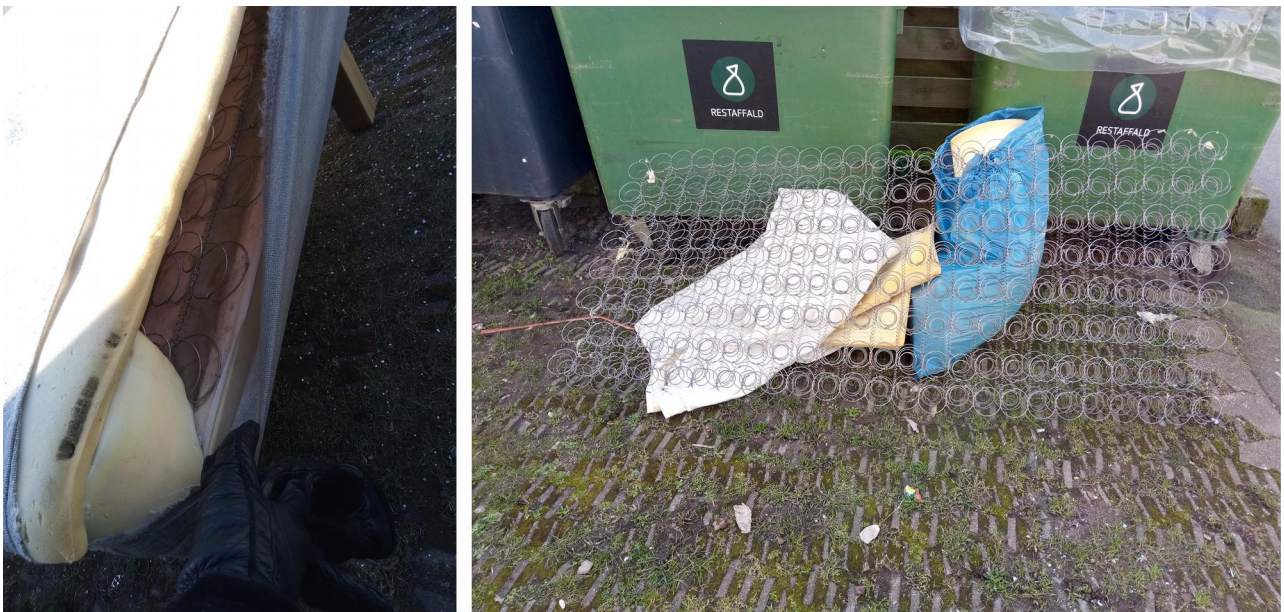
Figure 6.2: Discarded Bed – Materials permanently attached (left & middle) & Mattress disassembled into cover, springs and upholstery (Photos taken by author)
