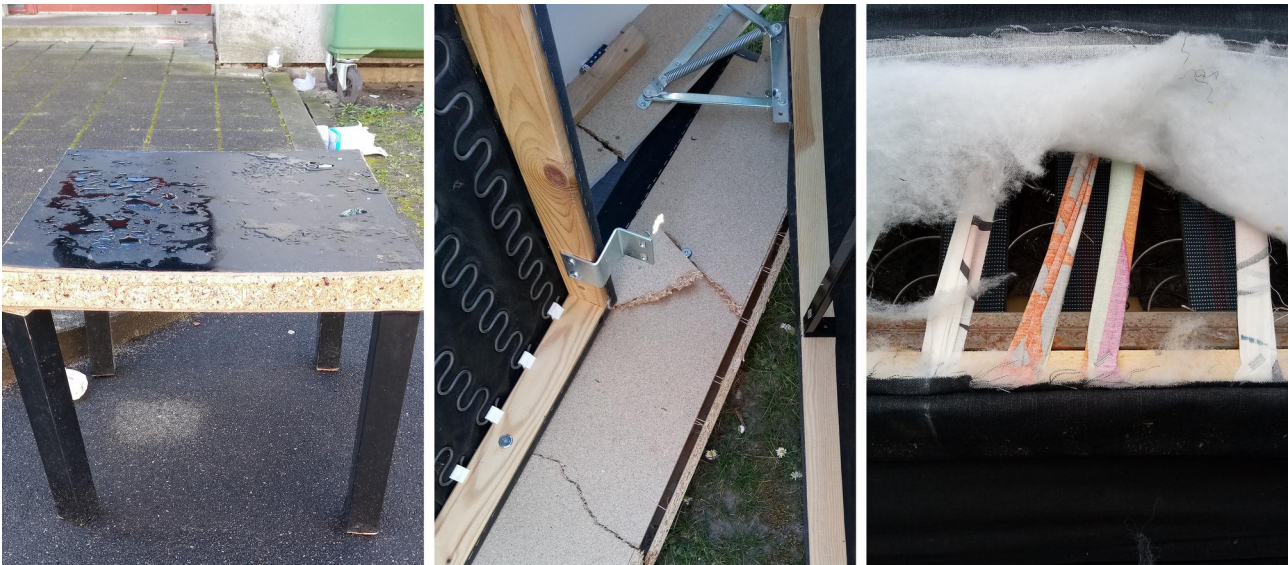
Figure 6.1: Discarded Products: Coffee-table from laminated chip-board (left); Sofa made from Particle-board with material-breakage (middle) & Sofa made from multiple materials (right) (Photos taken by author)
