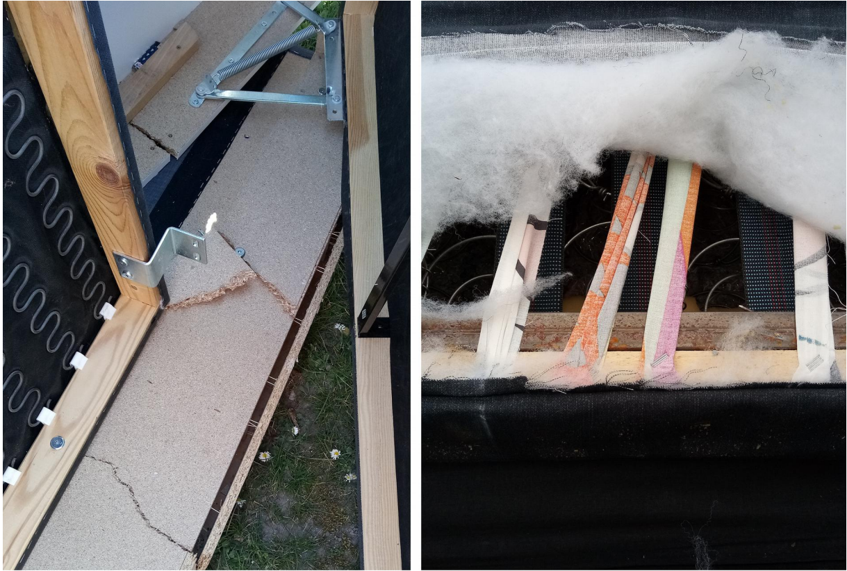
Figure 6.1: Discarded Products: Sofa made from Particleboard with material-breakage (middle) & Sofa made from multiple materials (right) (Photos taken by author)
