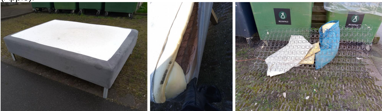
Figure 6.2: Discarded Bed – Materials permanently attached (left & middle) & Mattress disassembled into cover, springs and upholstery (Photos taken by author)
