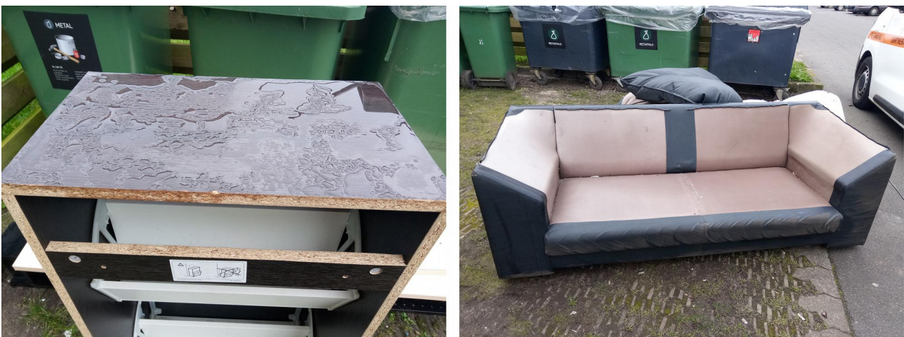
Figure 5.16: Furniture Exposed to Rain - Shelf from MDF & Leather couch (Photos taken by author)
