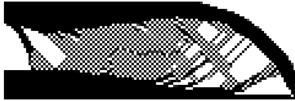
Figure 2.6. Checkerboard pattern formation when solving the MBB problem.
