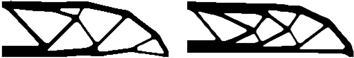
Figure 5.2. Left: a volume minimization MBB-problem subject to a compliance constraint solved with regular continuation of the \beta -variable. The resulting volume fraction is 0.340 and measure of nondiscreteness M_{nd} = 0.004 . Right: the same problem solved with adjusted MMA asymptotes and no continuation. Resulting volume fraction is 0.406 and M_{nd} = 0.01 . The eventual discreteness parameter is \beta_{lim} = 256 in both cases, and the volume preserving threshold filter is used with \eta = 0.5 .
