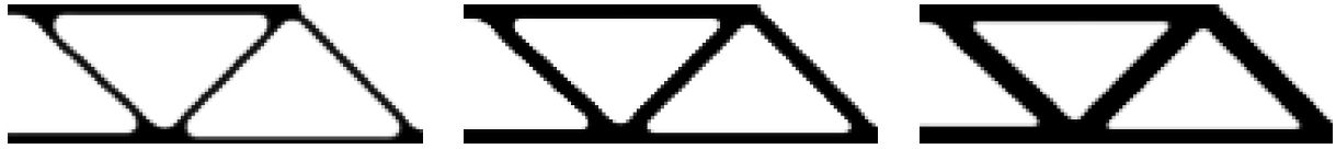
Figure 2.16. Results of minimizing volume subject to a compliance constraint on the MBB-beam using robust TO. From left: eroded ( \eta = 0.75 ), intermediate ( \eta = 0.5 ) and dilated ( \eta = 0.25 ) designs.
