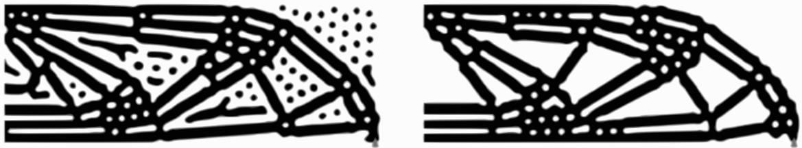
Figure 7.2. Maximum and minimum length scale imposed on both solid and void (left) and on solid only (right). Figure from Lazarov and Wang [2017] .
