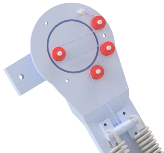
Figure 4.14: Detailed view of the pulley system.
