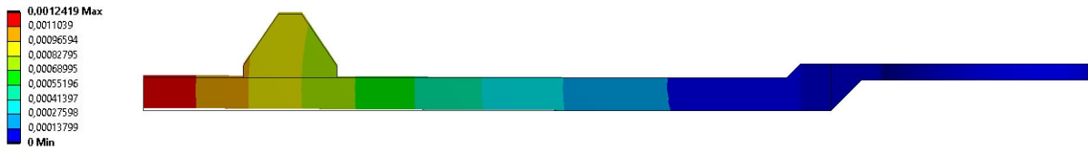
Figure 6.5: Maximum total deformation of the initial design subjected to load case 1. The color bar is given with the unit meter.
