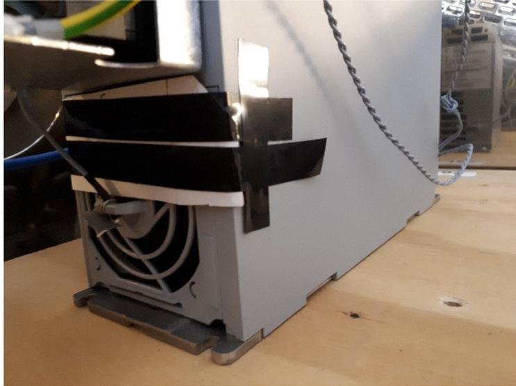
**Figure 4.2:** Photograph of the FC302 drive with a partially blocked (slightly under 50%) air passage.
