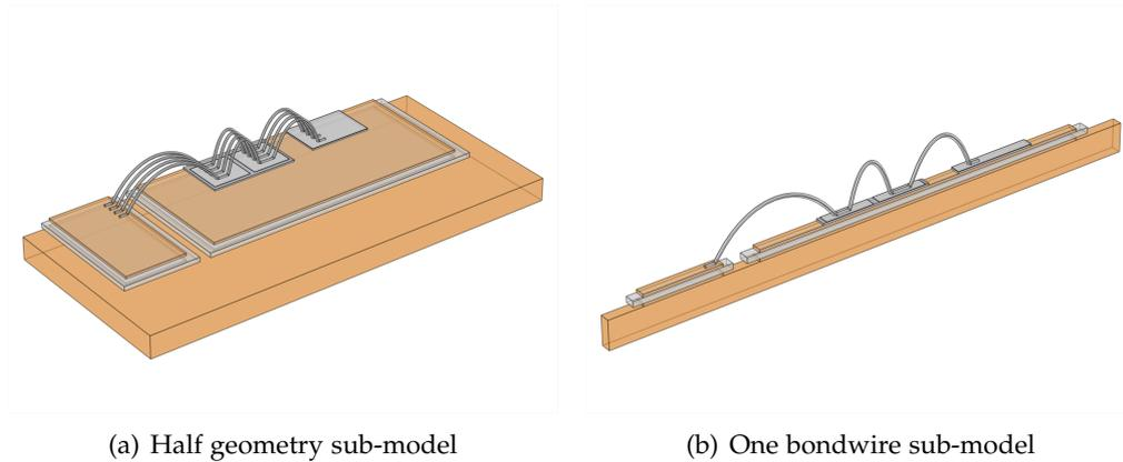
**Figure 4.3:** IGBT sub-model
