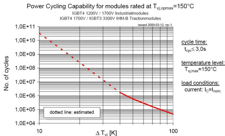
**Figure 2.1:** IGBT power module Power cycling capability graph, taken from Infineon FP50R06KE3. On the horizontal axis is the variation of the junction temperature between on an off-state of the module. On vertical axis is the number of cycles to failure
