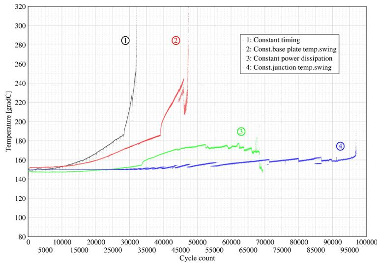
**Figure 2.5:** Evolution of maximum junction temperature for all four different control strategies during PC. Taken from [4]
