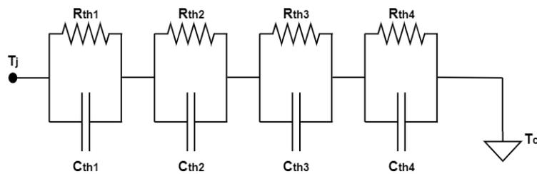
Figure 2.4: Foster Model of Infineon FP50R06KE3, with its partial thermal resistances and its corresponding thermal capacitances.
