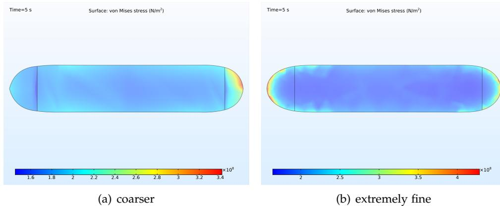
**Figure 4.2:** Stress distribution result with different mesh sizes
