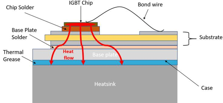
Figure 2.2: Heat generation in IGBT modules
