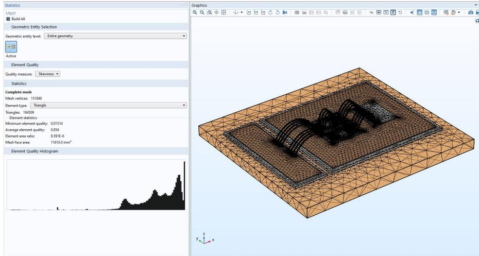
**Figure 4.1:** Mesh statistics and the associated mesh used in the simulation
