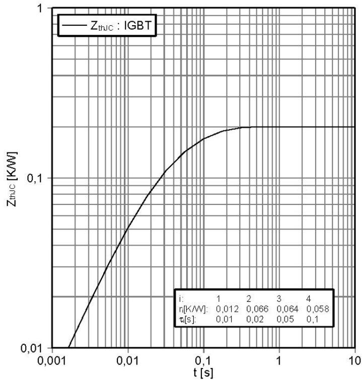
Figure 2.3: Transient thermal impedance (Infineon FP50R06KE3)
