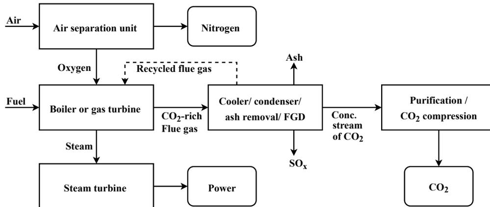
Figure 46: Oxyfuel-combustion carbon capture process. Adapted from (Wall, 2007).
