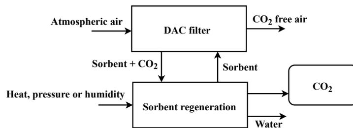
Figure 50: Showing DAC system from Climeworks. Adapted from (Azarabadi & Lackner, 2019).
