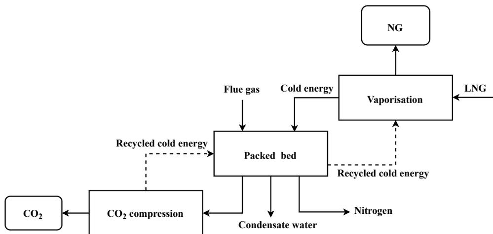
Figure 49: Cryogenic packed bed CO<sub>2</sub> capture with LNG vaporisation. Adapted from (Song et al., 2019). Note: The figure is simplified as one packed bed, however it is possible operating the system as dynamically in several beds.
