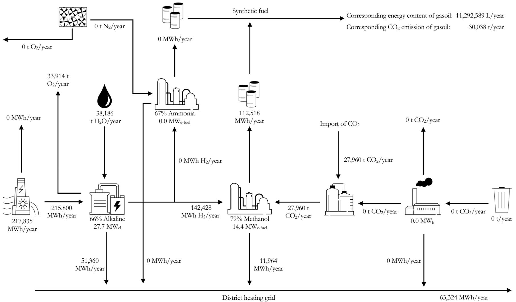
Figure 23: Flow diagram of PtX system from Johan Dabl Land producing methanol.
