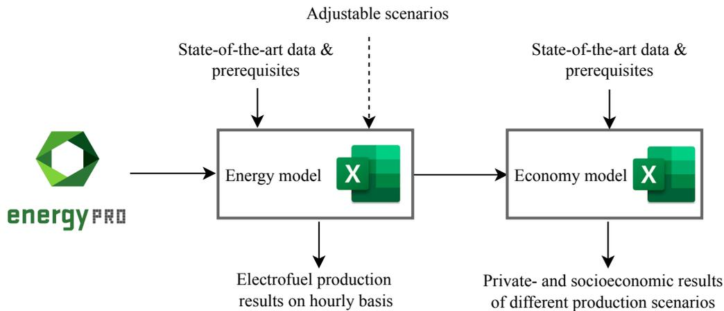
Figure 4: The techno-economic model for analysing different alternatives of electrofuel production.
