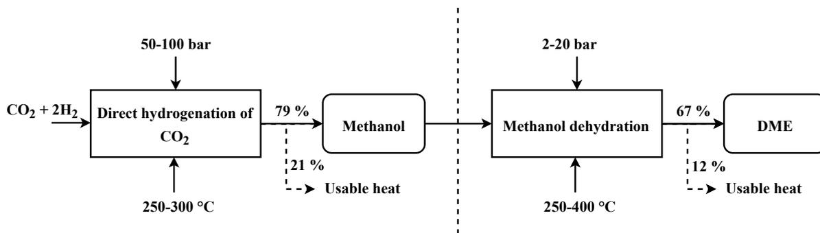
Figure 8: Production of DME from methanol dehydration.
