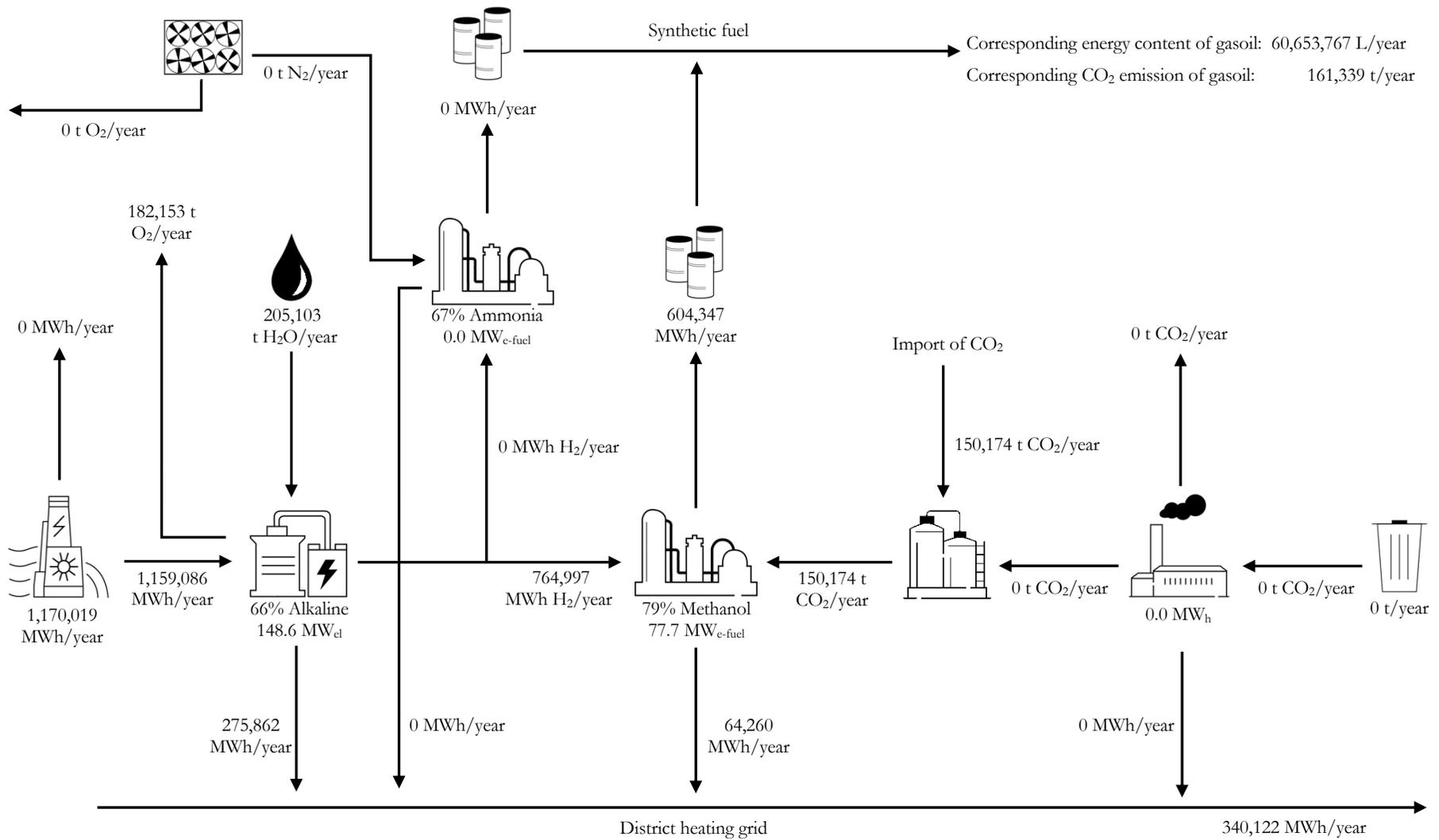
Figure 30: Flow diagram of PtX system from Imarsuup Isua producing methanol.
