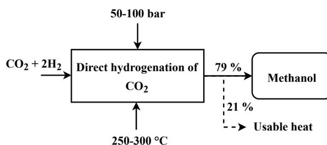
Figure 7: Methanol production from direct hydrogenation of CO<sub>2</sub>.
