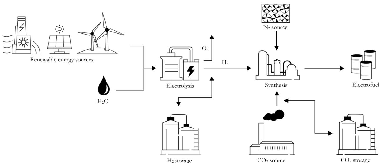
Figure 5: Simplified diagram of electrofuel production process.
