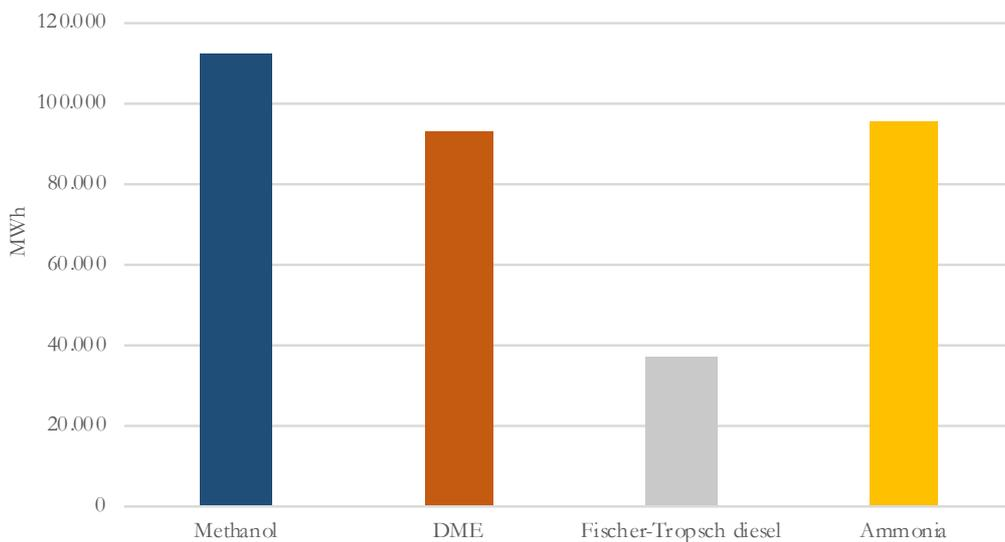
Figure 22: Carbon-based fuel productions based on imported CO<sub>2</sub> and ammonia based on captured N<sub>2</sub> from ambient air.
