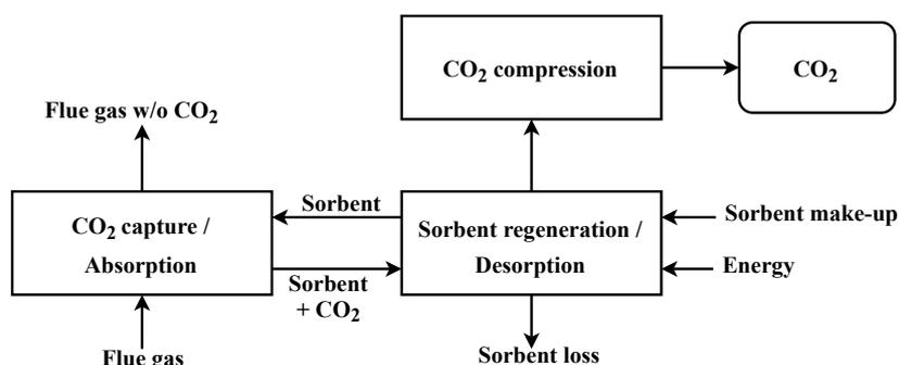
Figure 6: Absorption and desorption process. Adapted from Utgard (2007); Song et al. (2019).
