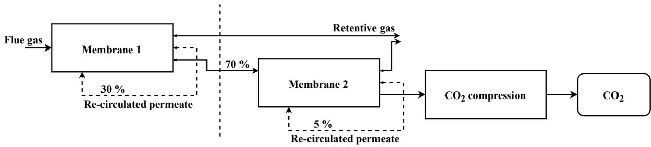
Figure 48: Membranes CO<sub>2</sub> capture with recycled permeate. Adapted from Song et al. (2019).
