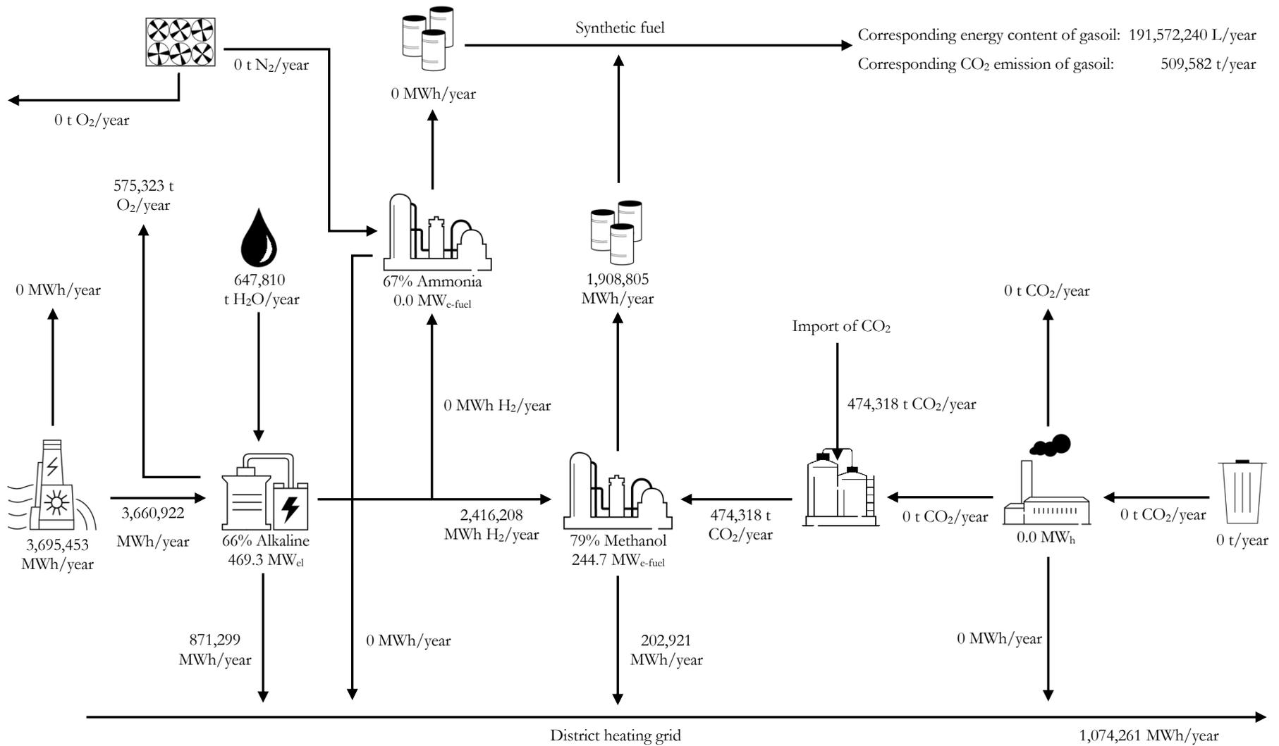
Figure 36: Flow diagram of the PtX system from Tasersiaq producing methanol.
