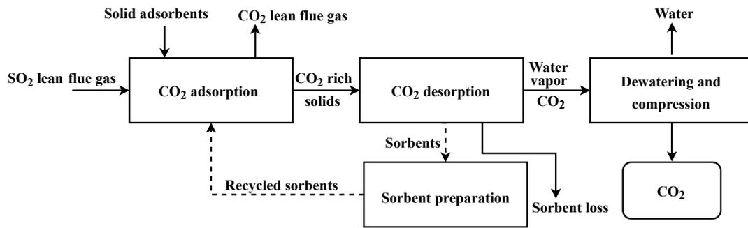
Figure 47: CO<sub>2</sub> adsorption and desorption process. Adopted from Glier and Rubin (2013).
