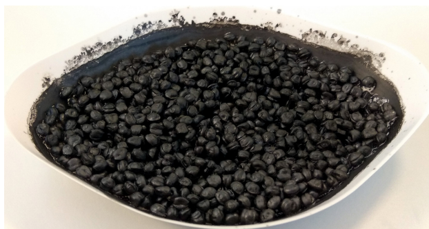
Fig. 5.2 Polymer beads coated with graphene (bads were originally semi-translucent white).
