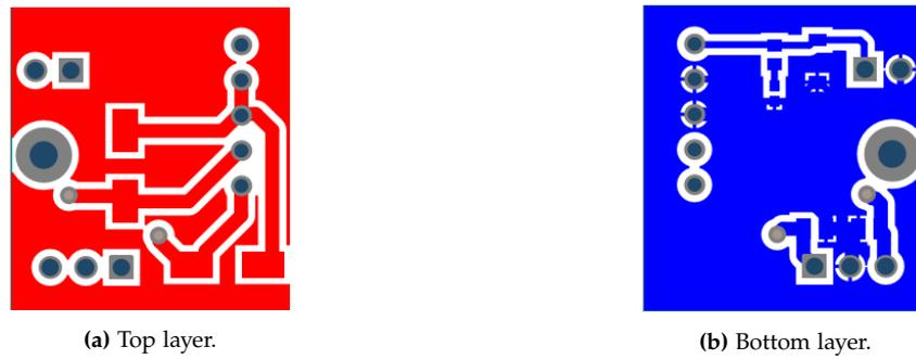
Figure B.5: Current sensor PCB layout.
