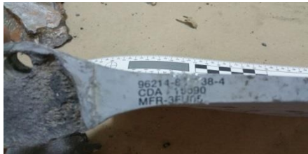
Figure X GBU-12 Paveway II guidance unit wing fragment showing manufacturer's Commercial and Government Entity code 3FU05 135
