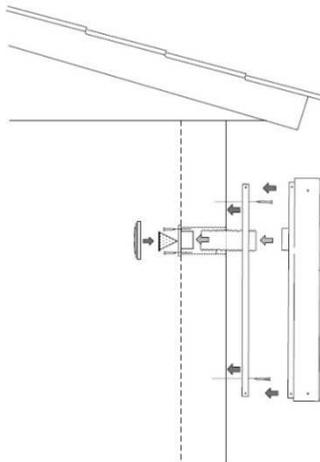
Figure 1.2.2.2 Installation collector of the wall
