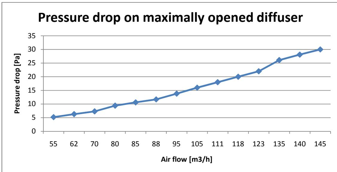
Figure 3.3.1.2: Pressure drop on flex pipe with maximally opened diffuser
