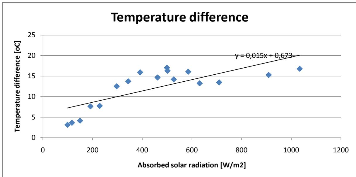
Figure 6.1.1: Equation for temperature difference
