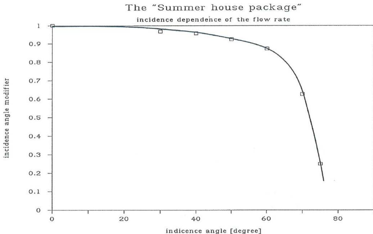
Figure 1.4.1.4 The influence of the incidence angle on the efficiency
