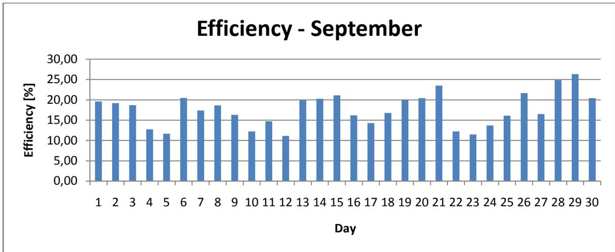
Figure 10.4.9: Monthly performance of the collector – efficiency in September
