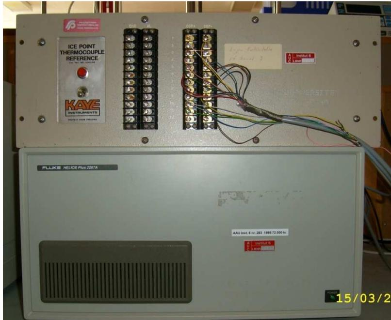
Figure 9.1.1.3: Fluke Helios Plus 2287A Data Logger with Ice Point Thermocouple Reference
