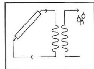
Figure 1.1.2.6 Type 6 solar air collector
