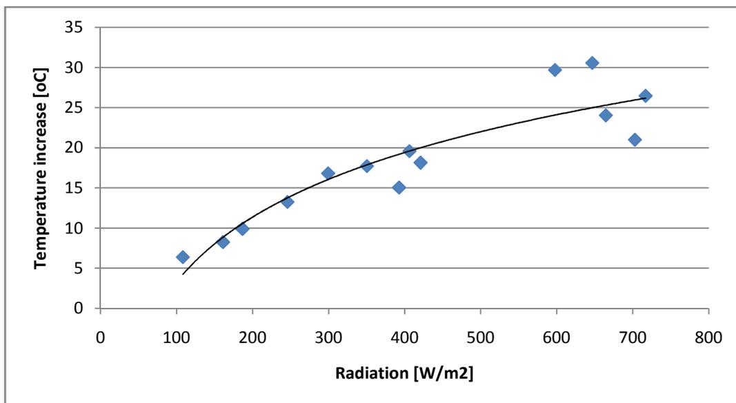
Figure 4.1.4: Dependence of the temperature increase from the solar radiation
