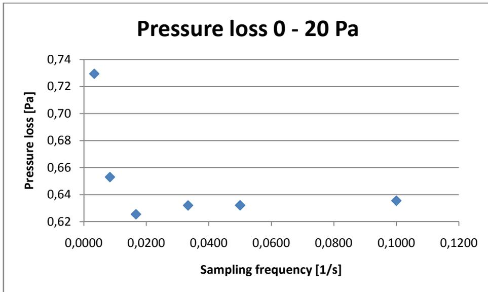
Figure 3.2.2: Average results for pressure loss with different sampling frequency
