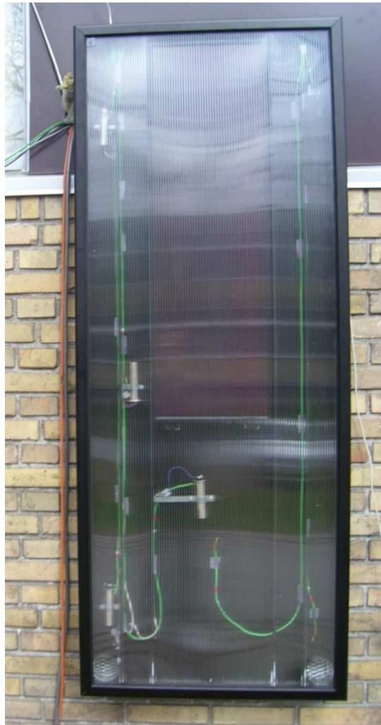
**Figure 3.1.1:** Picture of the collector with thermocouples mounted inside
