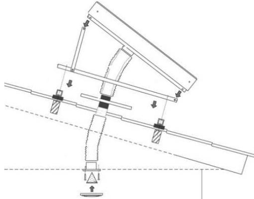
Figure 1.2.2.1 Installation of the collector on the roof
