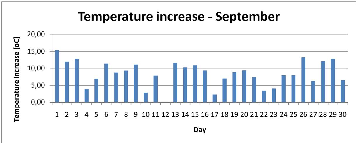
Figure 10.2.9: Monthly performance of the collector – temperature increase in September
