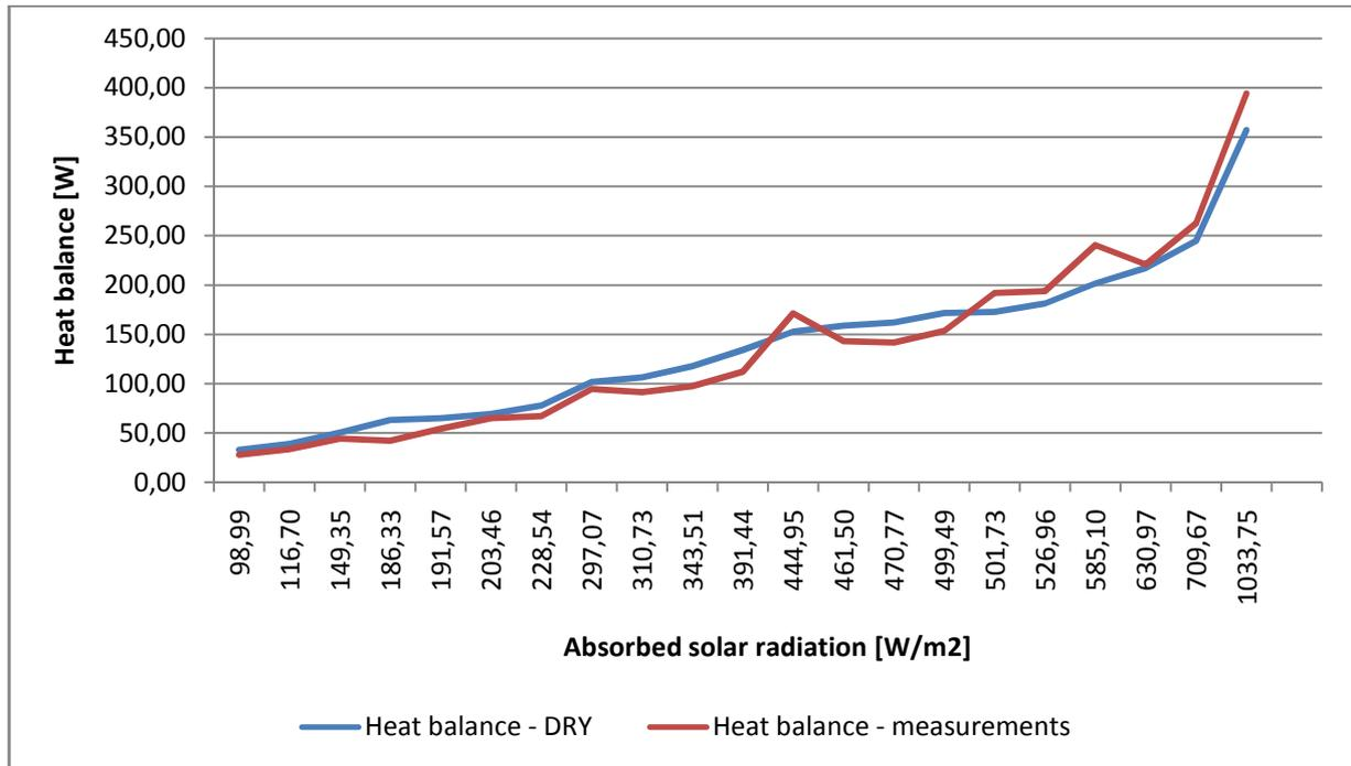
**Figure 6.6.1: Comparison of heat balance from DRY file and measurements in reference to absorbed solar radiation**
