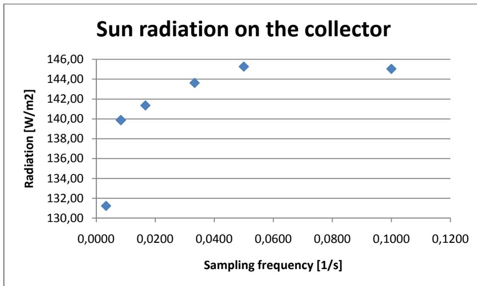
Figure 3.2.4: Average results for sun radiation on the collector with different sampling frequency
