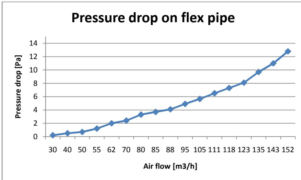
Figure 3.3.1.1: Pressure drop on the flex pipe.
