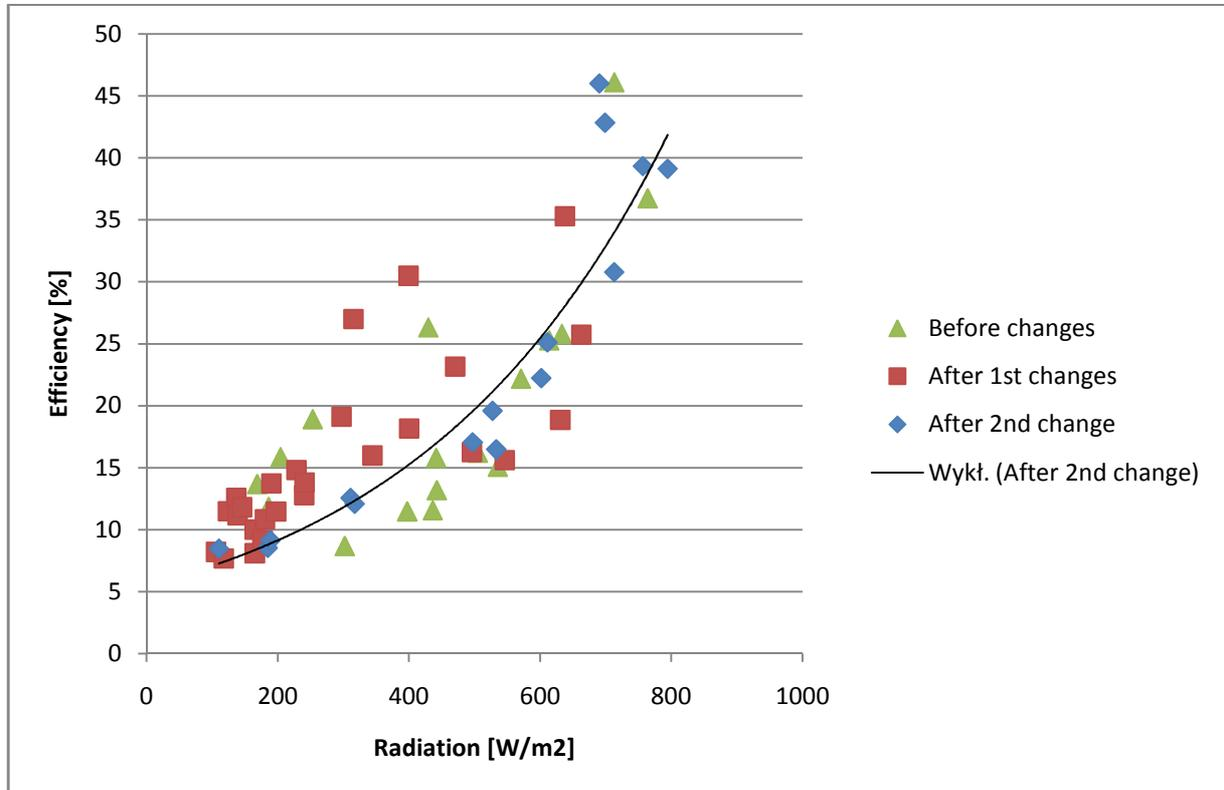
Figure 5.2.4: Efficiency dependent from radiation in three cases
