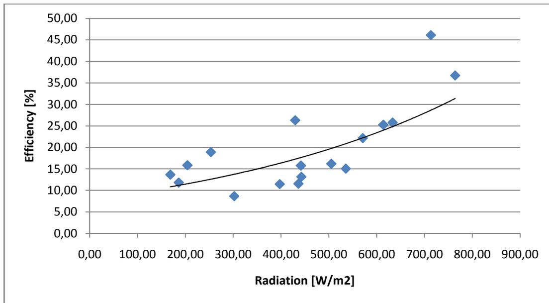
Figure 4.3.4: Dependence of the efficiency from the solar radiation
