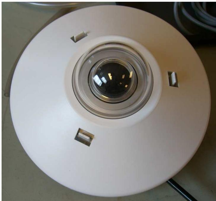
Figure 9.2.1.2: Pyranometer CM21
