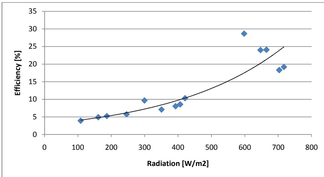
Figure 4.1.5: Dependence of the efficiency from the solar radiation
