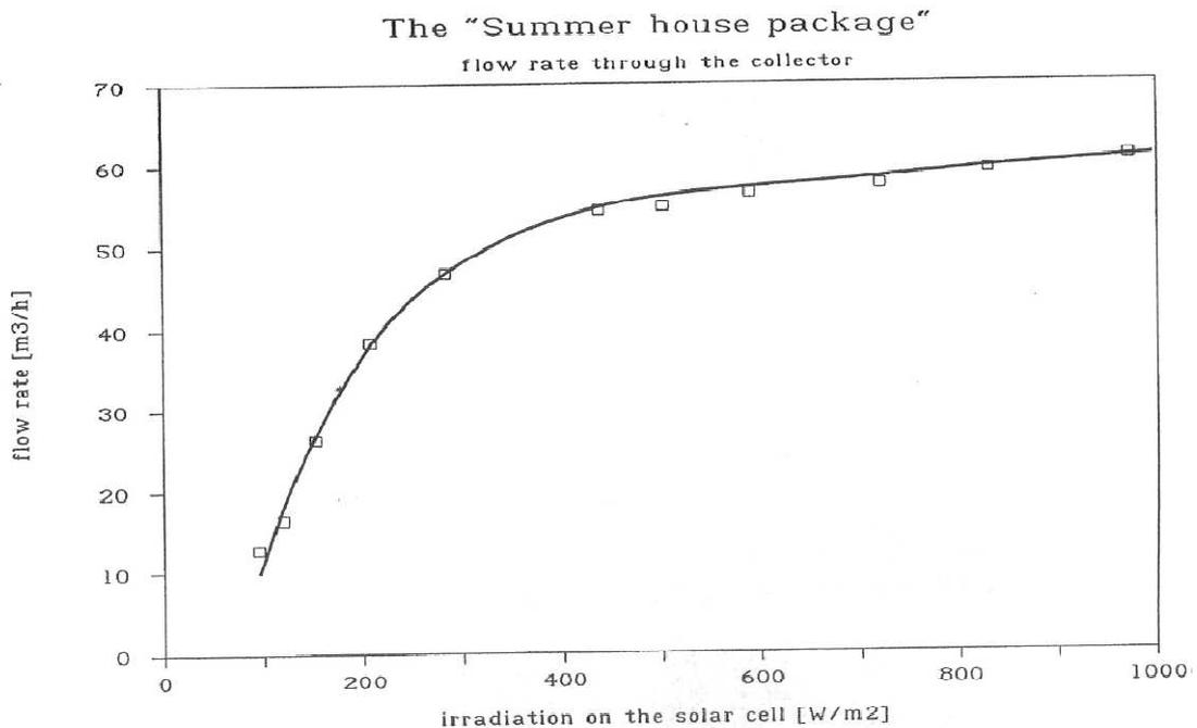
Figure 1.4.1.3 The flow rate through the air solar collector dependent on the radiation on the solar cell panel
