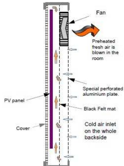
Figure 1.3.1.1 SolarVenti air collector
