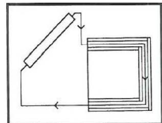
Figure 1.1.2.3 Type 3 solar air collector
