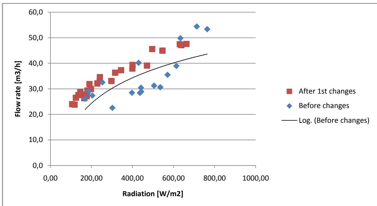
Figure 5.1.2: Flow rate dependent from radiation in two cases
