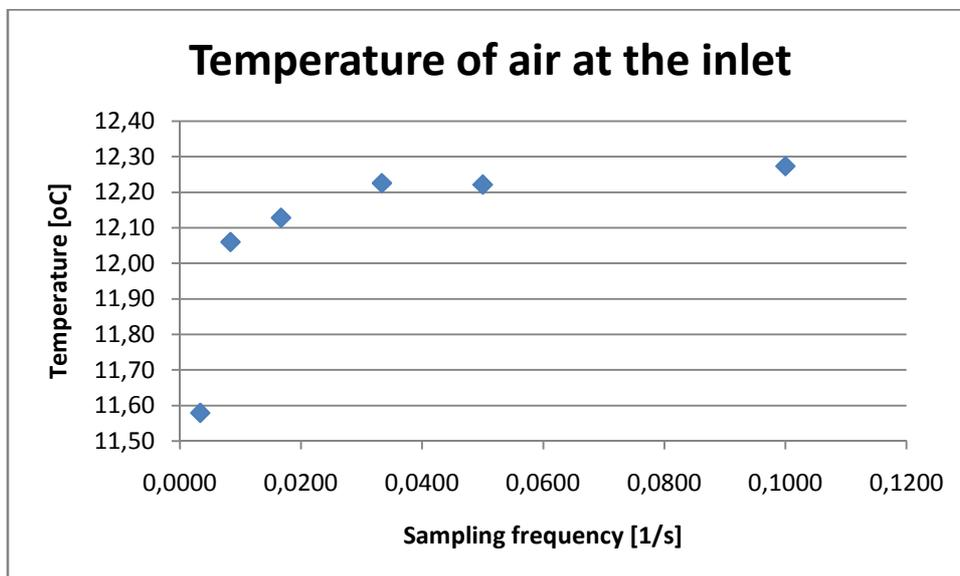
**Figure 3.2.1: Average results for temperature of air at the inlet with different sampling frequency**
