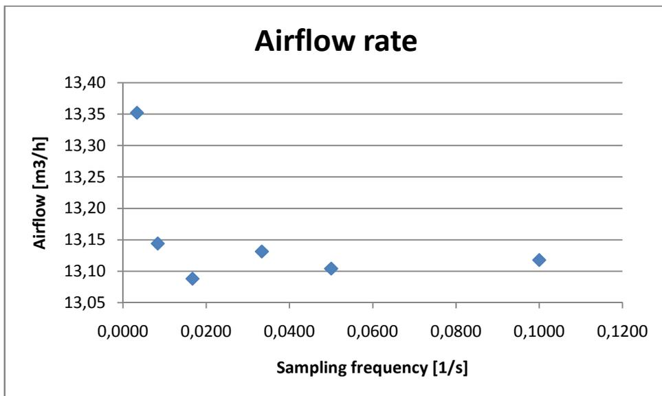
Figure 3.2.3: Average results for airflow rates with different sampling frequency
