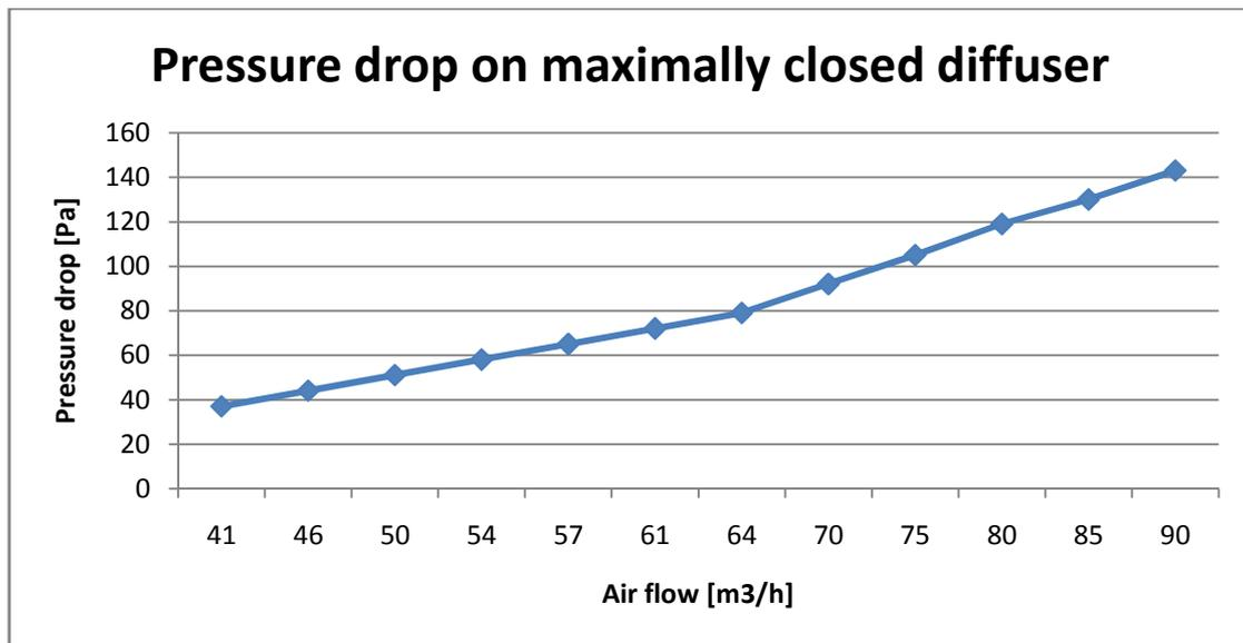
Figure 3.3.1.3: Pressure drop on flex pipe with maximally closed diffuser
