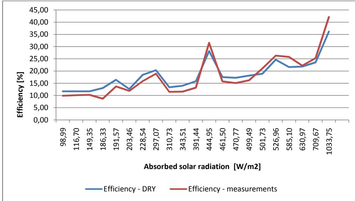
**Figure 6.6.3: Comparison of efficiency from DRY file and measurements in reference to absorbed solar radiation**
