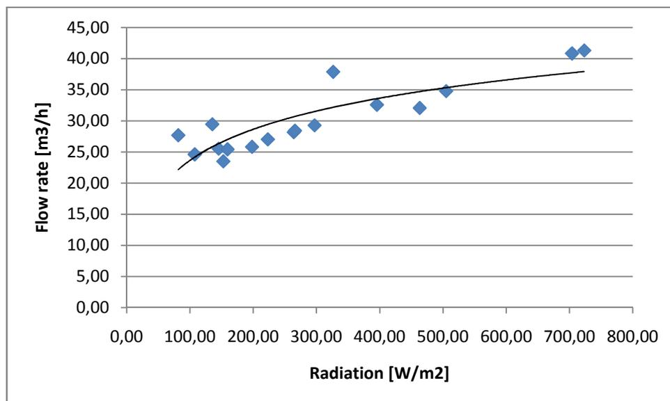
Figure 5.3.2: Flow rate dependent from radiation in case of reverse fan
