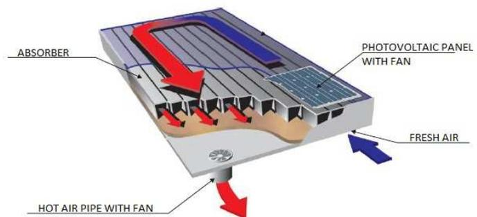
Figure 1.3.1.2 Twin and Top Solar air collector
