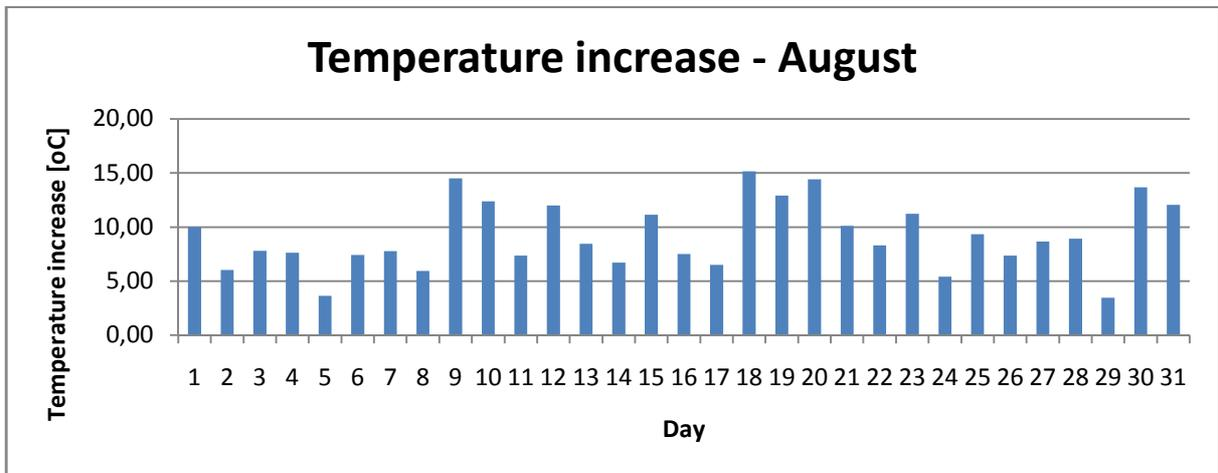
Figure 10.2.8: Monthly performance of the collector – temperature increase in August
