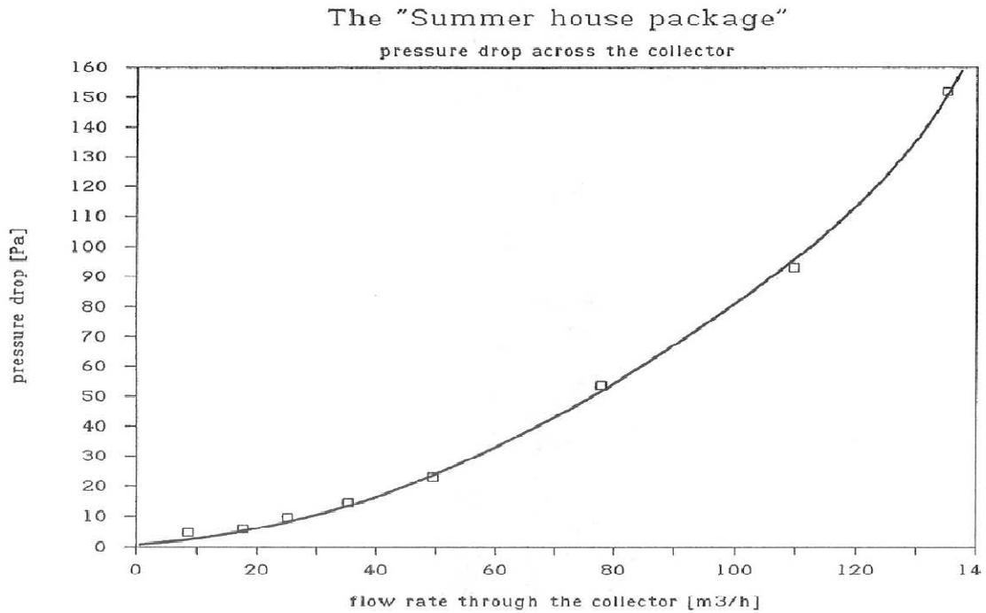
Figure 1.4.1.2 The pressure drop across the solar air collector of the Summer House Package (including 30 cm of flexible duct) dependent on the air flow through the collector
