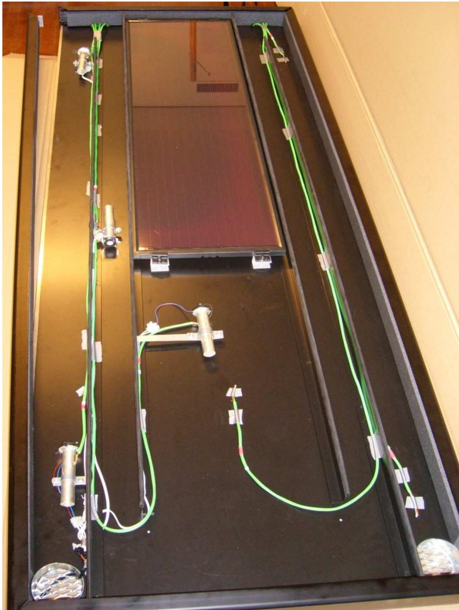
**Figure 3.4.1: Position of the thermocouples**
