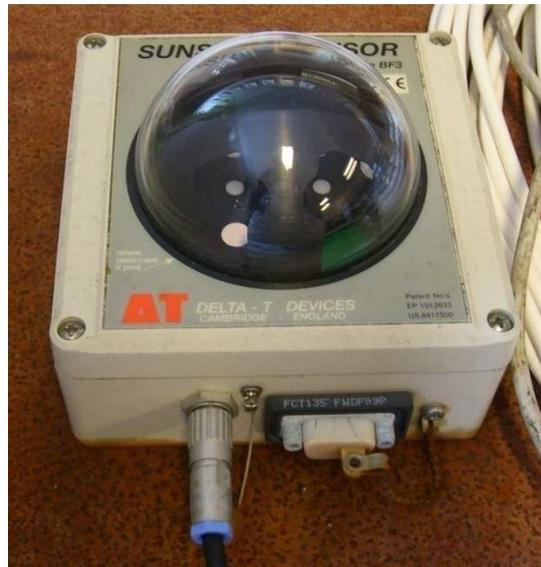
**Figure 9.2.1.3: Pyranometer BF3**
