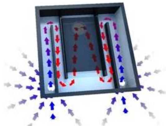
Figure 1.2.1.4 Air transfer in collector
