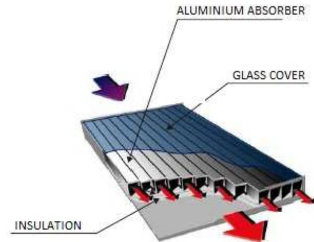
Figure 1.3.1.3 JumboSolar air collector
