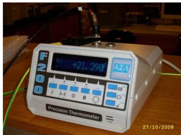
Figure 9.1.2.2: Precision Thermometer F200
