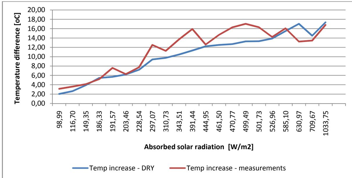
**Figure 6.6.5: Comparison of temperature difference from: DRY file and measurements in reference to absorbed solar radiation**
