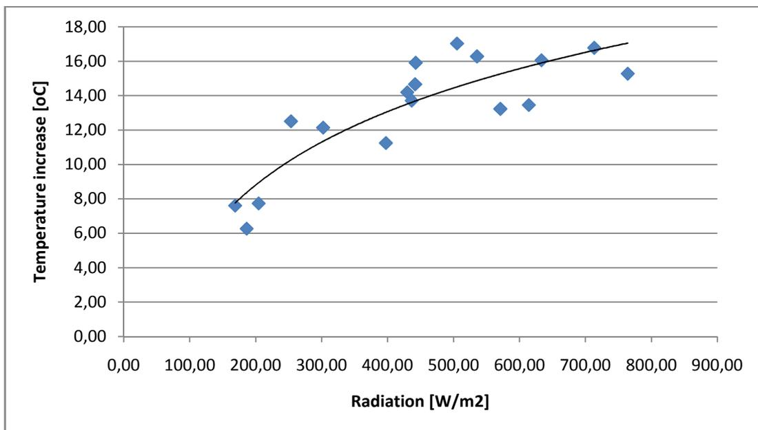
Figure 4.3.3: Dependence of the temperature increase from the solar radiation
