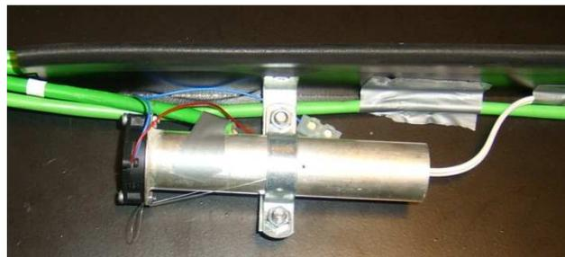
Figure 9.1.1.2: Thermocouples in silver coated shielding tube
