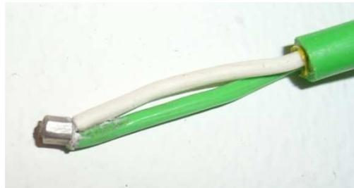
Figure 9.1.1.1: K-type thermocouple
