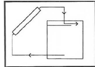
Figure 1.1.2.2 Type 2 solar air collector
