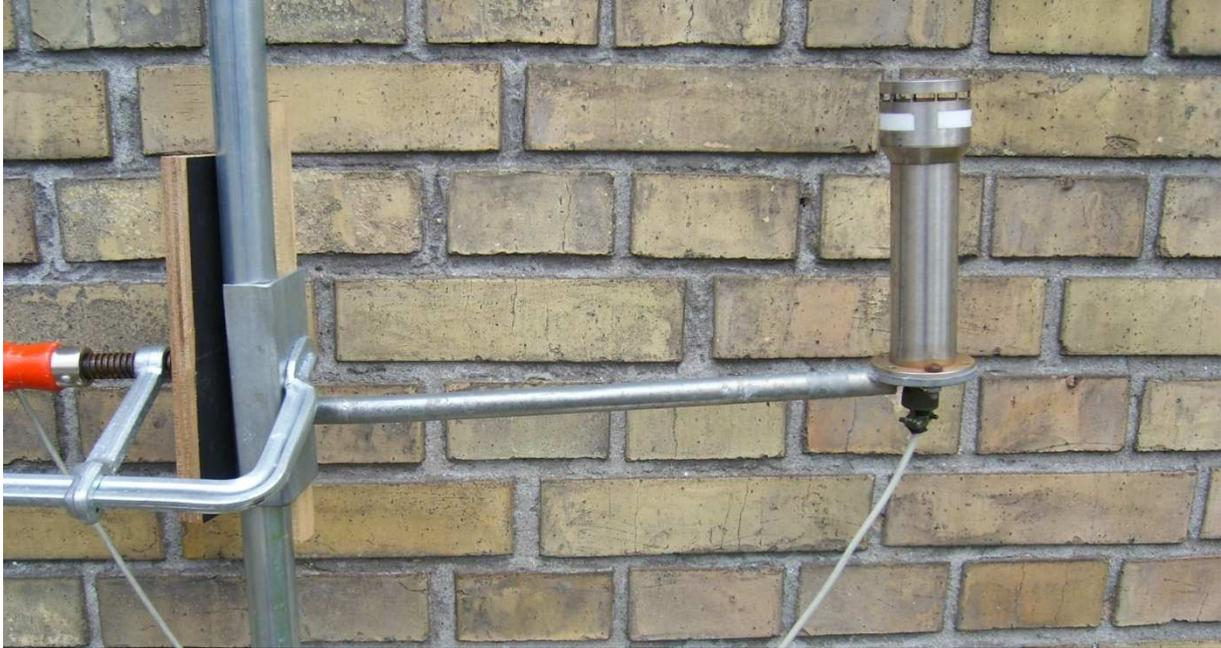
**Figure 3.8.2: Anemometer to measure local velocity.**
