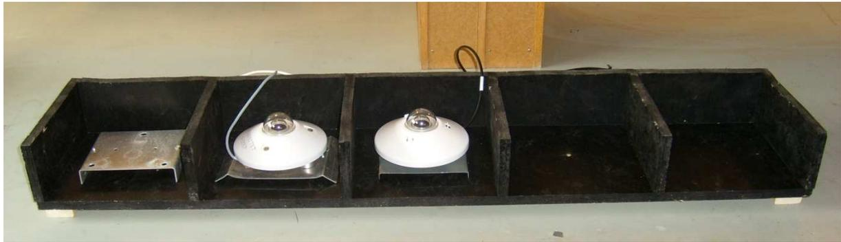
Figure 9.2.2.1: Setup for calibrating pyranometers
