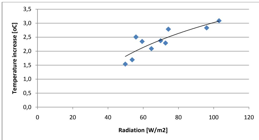
**Figure 4.2.2: Dependence of the temperature increase from the solar radiation**
