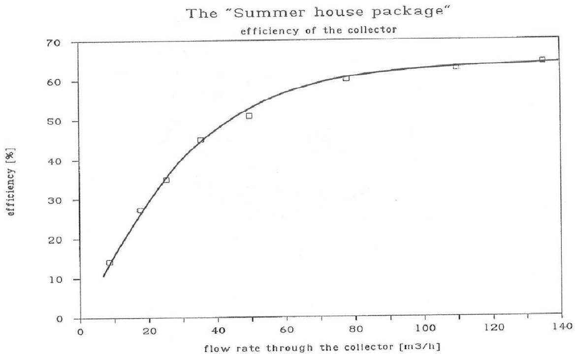
Figure 1.4.1.1 The efficiency of the air solar collector of the Summer House Package dependent on the air flow through the collector
