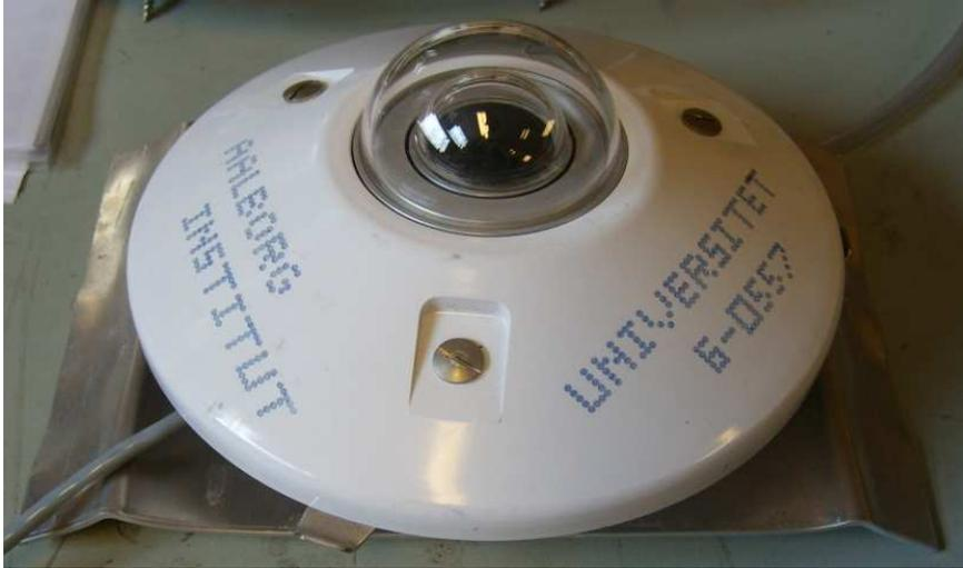
Figure 9.2.1.1: Pyranometer CM11
