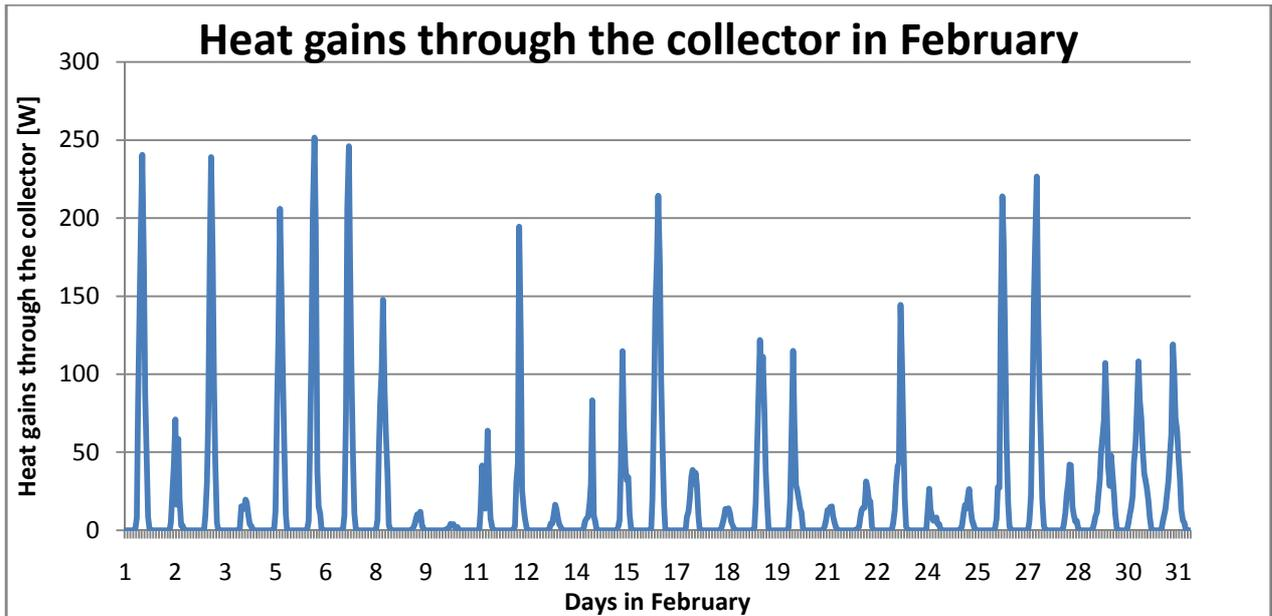
Figure 7.5.2.3: Results for heat gains through the collector in February
