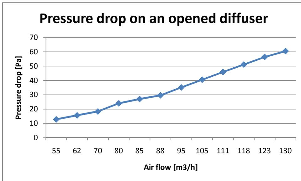
Figure 3.3.1.4: Pressure drop on flex pipe and diffuser in a middle position.
