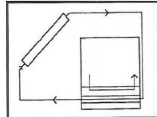
Figure 1.1.2.5 Type 5 solar air collector
