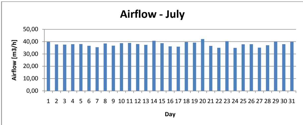
Figure 10.3.7: Monthly performance of the collector – airflow in July
