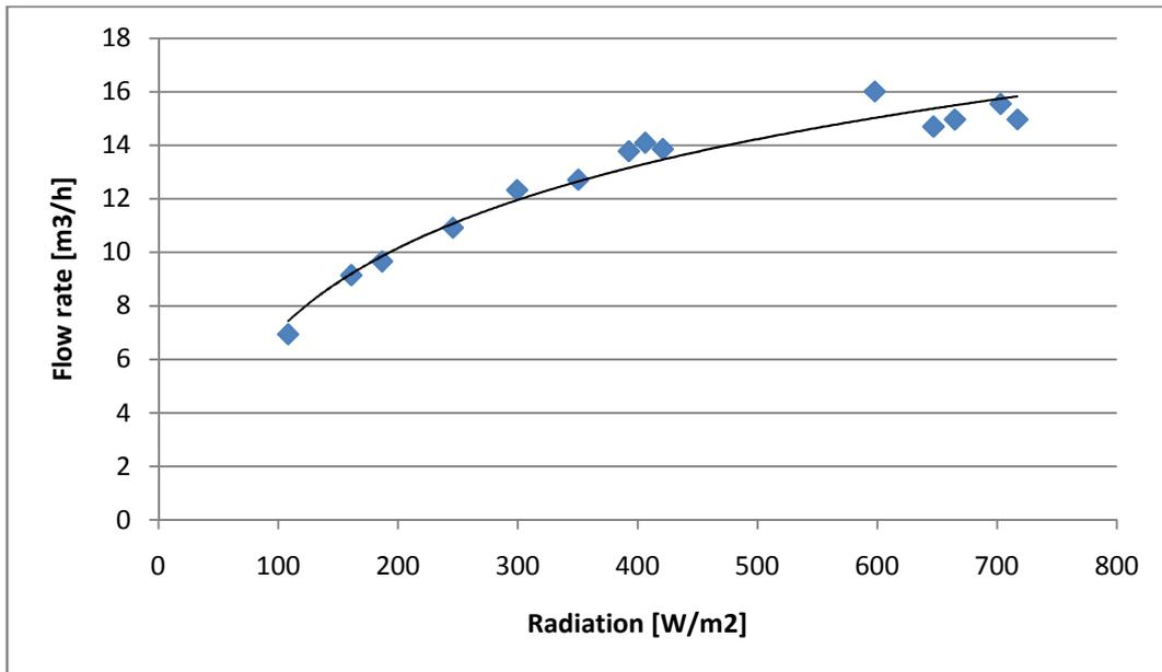
Figure 4.1.3: Dependence of the flow rate from the solar radiation
