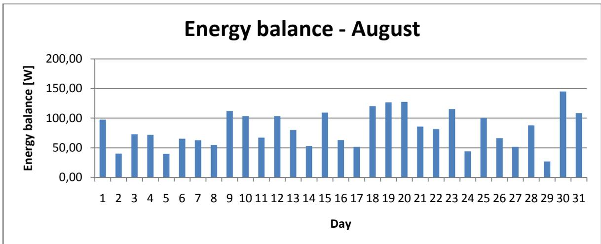
Figure 10.1.8: Monthly performance of the collector – energy balance in August
