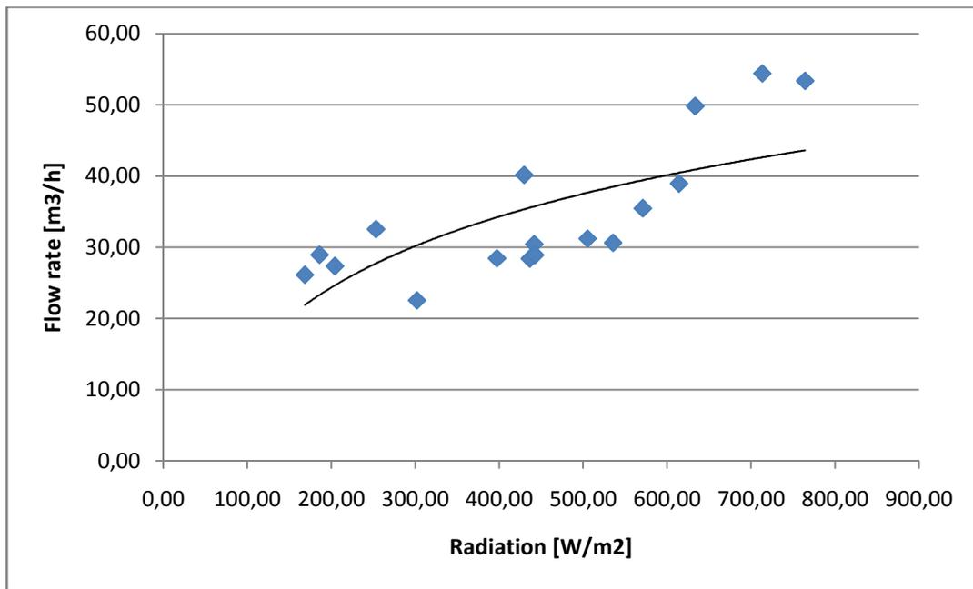
Figure 4.3.2: Dependence of the flow rate from the solar radiation
