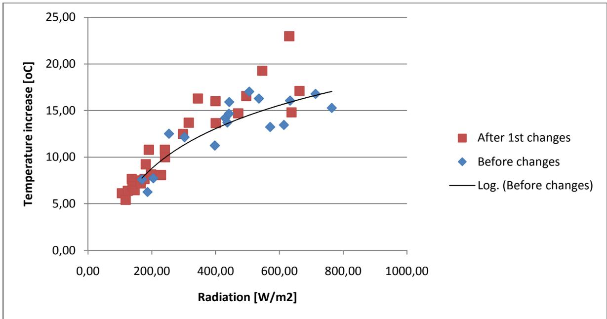
Figure 5.1.3: Temperature increase dependent from radiation in two cases
