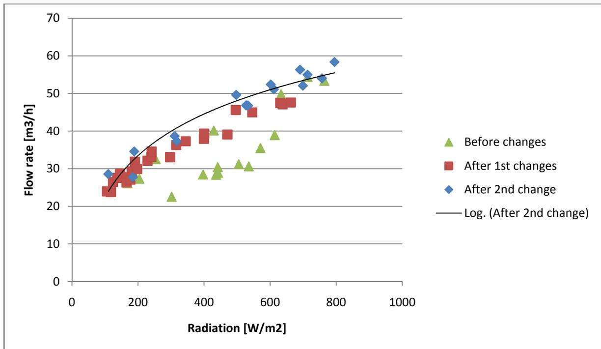
Figure 5.2.2: Flow rate dependent from radiation in three cases
