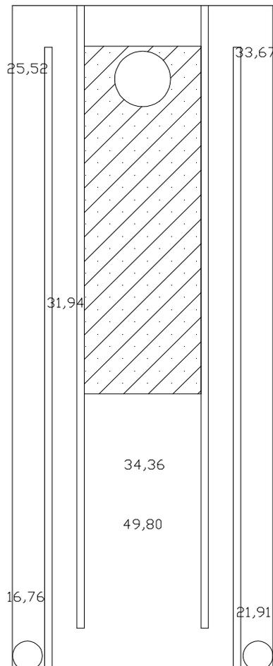
Figure 4.1.2: Collector with temperature distribution for an airflow equal to  $16,0 \text{ m}^3/\text{h}$
