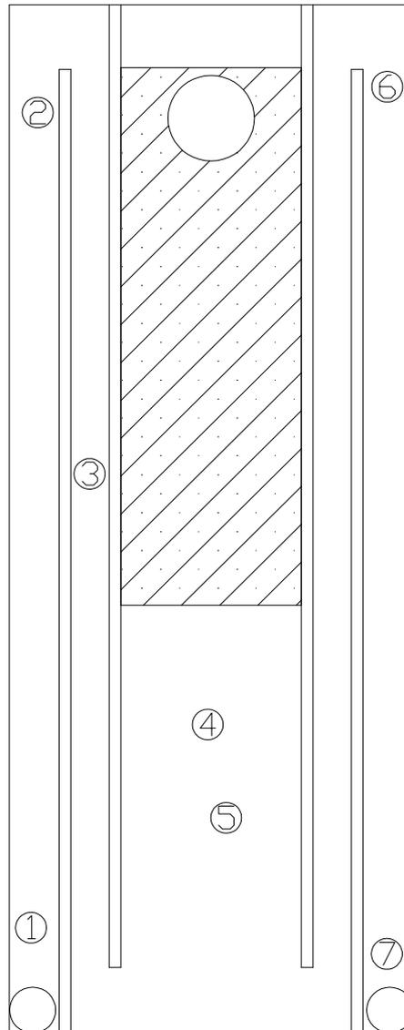
Figure 3.4.2: Position of the thermocouples on the collector
