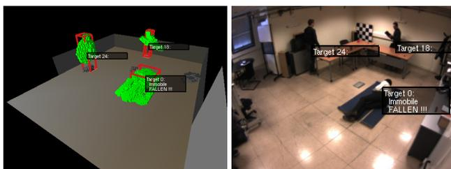
(a) Detected foreground is shown as green cubes, targets are shown using wire frame boxes, and info boxes are shown for each target. (b) Frame from one of the corner cameras with targets and info superimposed.
