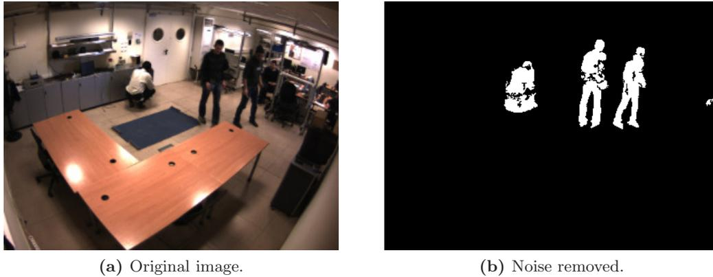
*Figure 4.11: Example of the final foreground mask after shadows and noise have been removed.*
