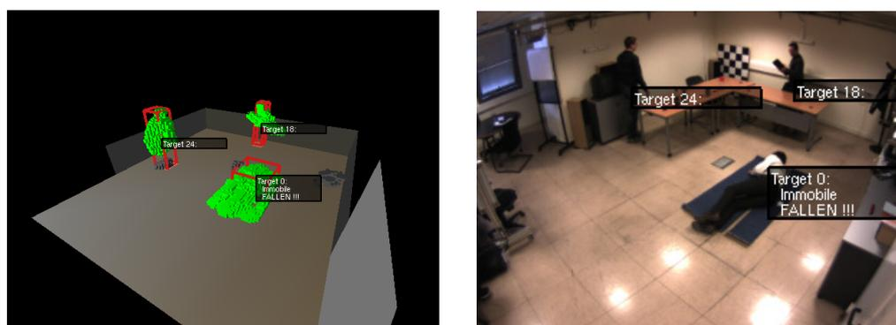
(a) 3D foreground with detected targets and reasoning results. Targets not shown as “immobile” have been classified as mobile. (b) Frame from corner camera with the same reasoning information as in (a).
