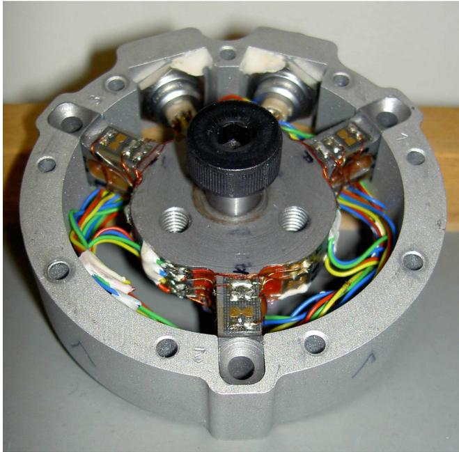
Figure 3.8: An image of the FTS sensor. The center part is connected to the leg, and the outer rim is attached to the foot. The three beams, that connects the center part with the outer rim, is bend or sheared slightly as a result of external forces.
