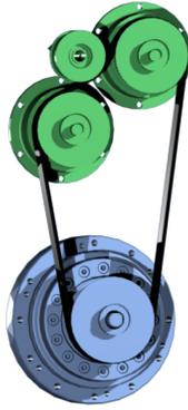
Figure 3.1: Gear setup, this is for one of the knees, two motors are connected to a belt with spur gears, the belt is connected to a harmonic drive gear.
