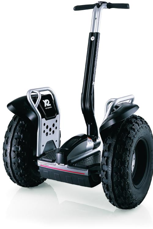
Figure 1.1: A picture of the X2 Segway, this is the commercial version of a classic control problem of balancing an inverted pendulum on a cart.
