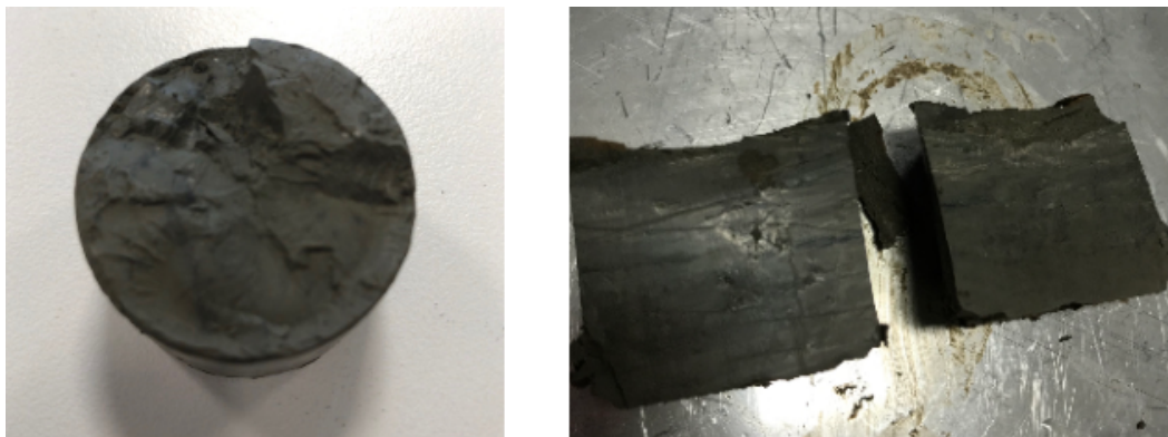
Figure 2.7: Sample from boring LH 830 used in Test03 before (left) and after (right) the consolidation test. (AAU lab)
