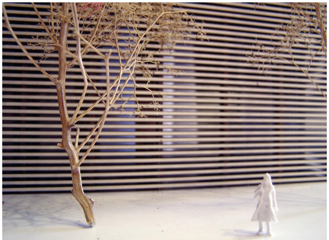
III. 277 The facade is constructed as a glass pane shaded by wooden lamellae.
