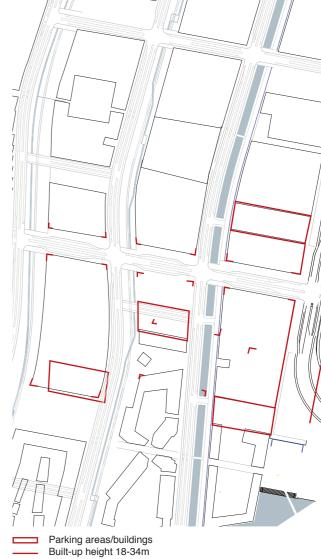
III. 132 1:5000. The overall parking plan constitutes areas for parking in Ørestad South. Around the corners of the buildings the height must be between 18-34m.
