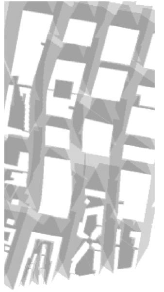
III. 135 Shadow diagram for June at 10-12-15 o'clock.
