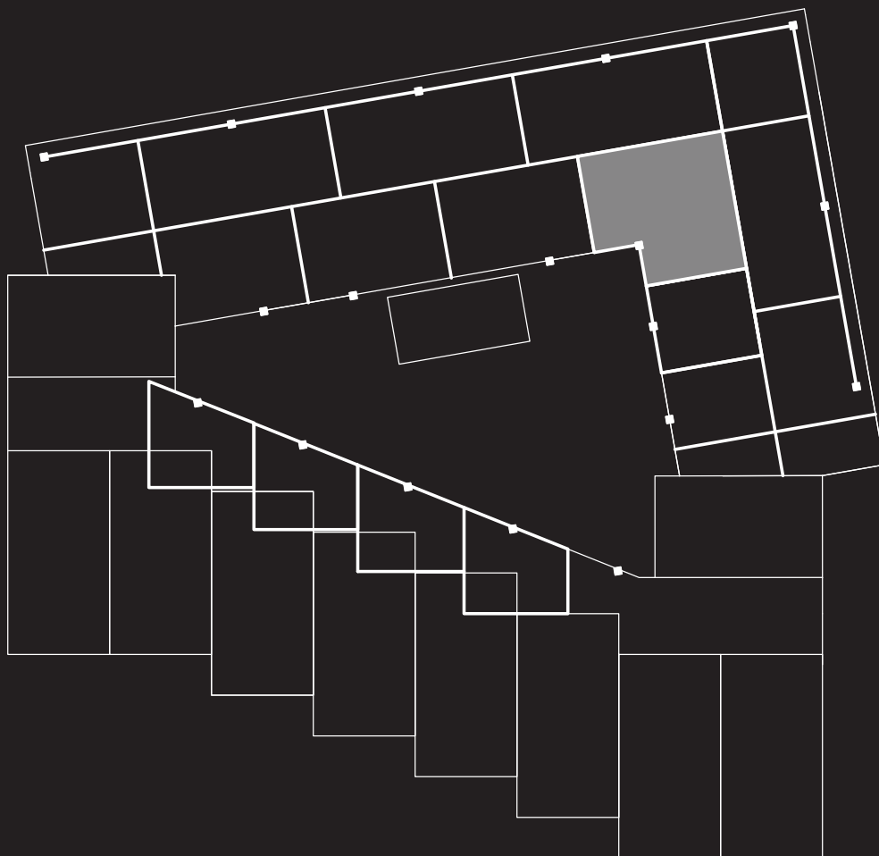
III. 03. Diagram showing the plan of the building and where the biggest line load is situated.
