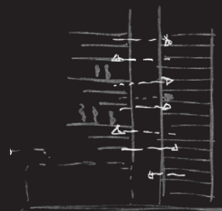
III. 103. The atrium as the buffer between the apartments and the offices. The atrium is the space that makes it possible to bring the two different functions together and eliminates the problem of having them joined in a vertical section.
