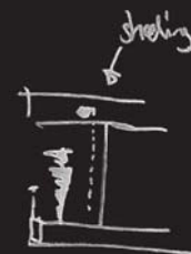
III. 146. The shading devise that is needed to avoid overheating of the apartments as calculated in BSim in p. 101 ill. 88.
