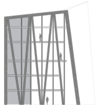
III. 101.3: Section showing how the plans are pulled in from the facade.
