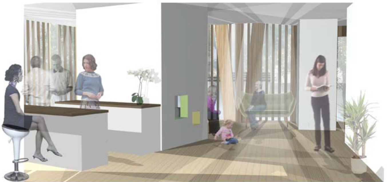
III. 135.2: View from the middle zone. The wooden facade and the floor gives a warm ambience, reflecting the light. The ceiling is of white acoustic plaster boards, and the walls stand in bright concrete, serving as thermal mass and bearing the floor plans.
